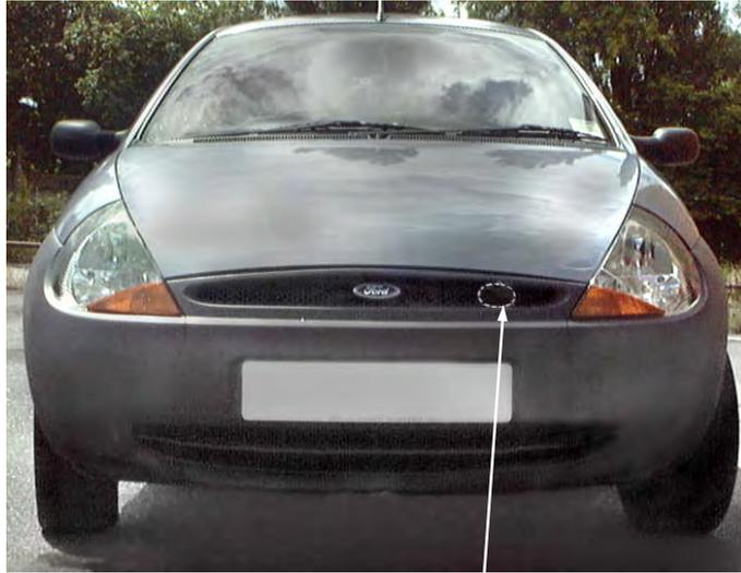
Feed the 60mm cold air hose to the front grille. Pierce / drill a 3mm hole in the end of the hose and secure to the grille using the long plastic ties supplied.
