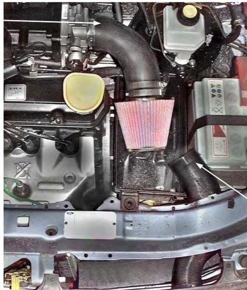
4. Insert half of the small plastic tube into the engine breather hose and secure with the original clip. Insert the tube into the hole in the base of the filter.
