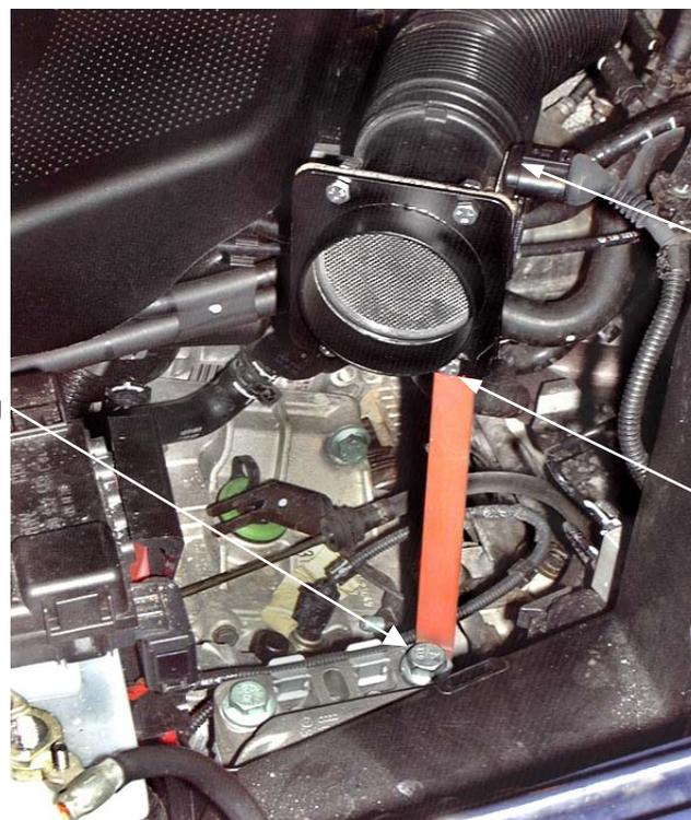
**2.** Refit the MAS to the intake hose and secure with the original hose clip. Reconnect the electrical harness plug.
