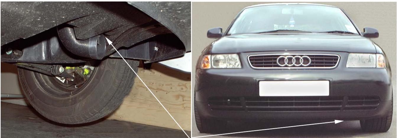
Feed the flexi cold air hose down to the undertray, drill pierce a 3mm hole in the end of the flexi cold air hose and undertray panel and secure with a long plastic tie supplied.
