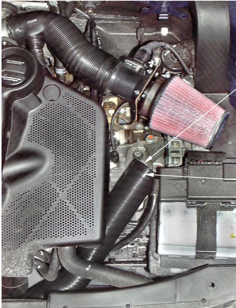
2. Carefully lengthen the flexi cold air hose to approx. 76cm / 30" and feed down to the front lower undertray. Secure the top of the hose to the original air box front support bracket using a long plastic tie supplied.
