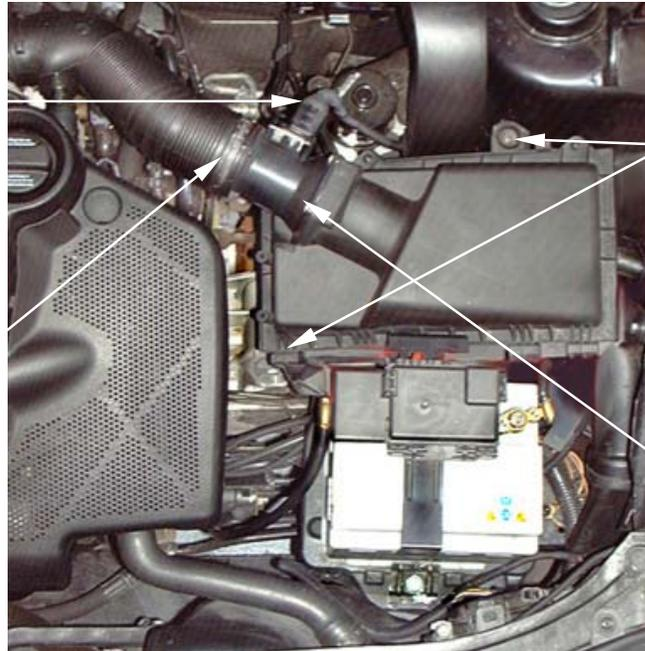
**3.** Remove the 2 securing screws from the air box assembly. Remove the complete air box from the engine bay.
