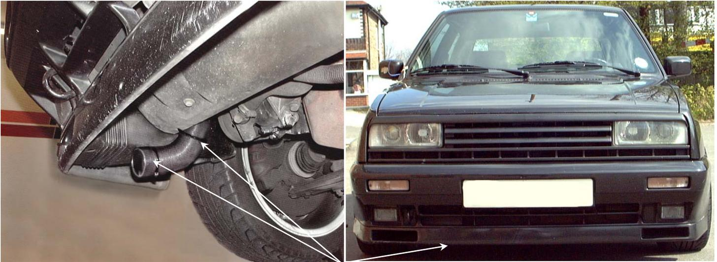
Taking all of the necessary safety precautions as per the manufacturers instructions, raise the front of the car. Feed the flexi cold air hose down to the lower spoiler then secure the hose away from the bottom drive pulley using a plastic tie supplied. Pierce / drill two 3 mm holes in the lower spoiler trim (or air ducting where fitted). Secure the front of the cold air hose using a long plastic tie supplied.
