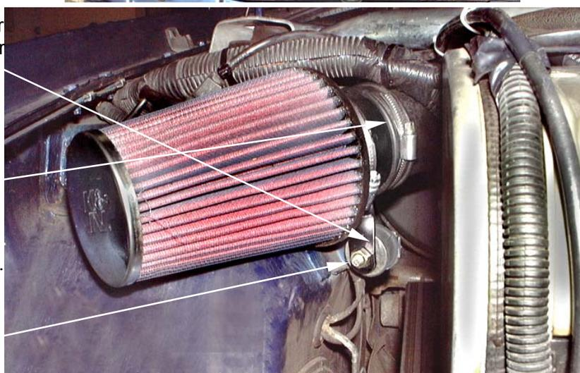
4. Attach the bracket the studded tube using the nuts and washers supplied.
