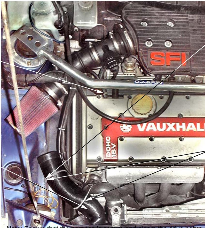
3. Attach the large 2 holed washer to the front air box mounting point using the original rubber mounting, nuts, 6mm spring washers and flat washer supplied. (The original rubber mounting bobbin can be located on the front of the air box.
