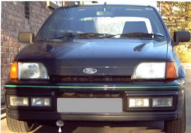
Feed the flexi cold air hose to the front lower spoiler and tie the hose to the metal cross member using one of the plastic ties. It may be advisable to ovalise the end of the hose to increase ground clearance.
