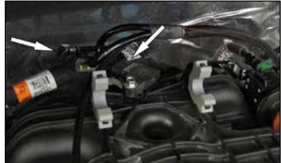
4. Connect the K&N® wiring harness to the MAP sensor and to the factory wiring harness. Route the K&N® wiring harness towards the driver's side inner fender. Secure the wiring harness with the provided tie wraps. Reinstall the decorative engine cover.
