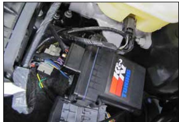
6. Connect the boost module wiring harness to the module and secure with the locking bolt.
