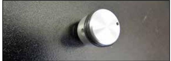
8. Find a suitable location to mount the sensitivity knob, drill a  $\frac{1}{4}$ "id hole, remove the knob and install the rheostat then reinstall the knob.
