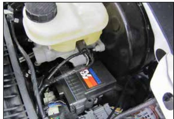
5. Mount the boost module in a suitable location such as under the brake master cylinder as shown using the provided tie wraps.
