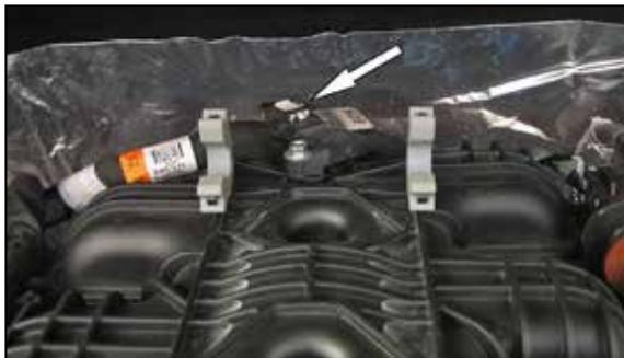
3. Remove the engine cover and then disconnect the MAP sensor electrical connection at the rear of the intake manifold.
