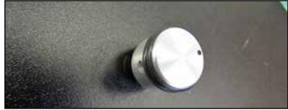
5. Find a suitable location to mount the sensitivity knob, drill a 1/4" id hole, remove the knob and install the rheostat then reinstall the knob.
