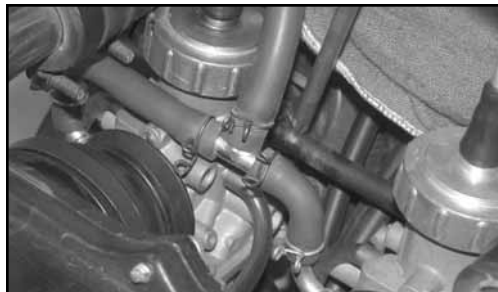
6. Remove all fuel lines from carburetors. It is recommended that you label each fuel line for ease of re-assembly. CAUTION: Be careful, fuel lines may still contain fuel.
