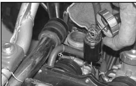
5. Loosen the cap on the slide assembly and remove from the carburetors.
