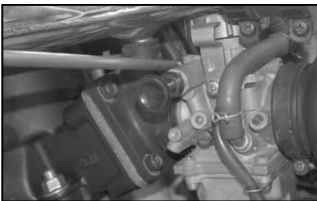
4. Loosen clamps that connect carburetors to the air box and the engine.
