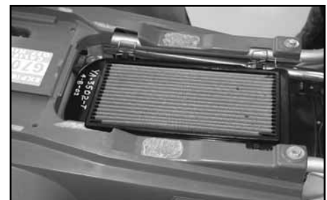
14. Install the X-STREAM™ POWERLID™ on to the air box using the stock retaining clips.
