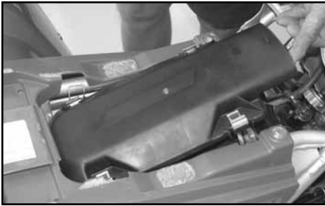
2. Unclip the air box retaining clips on lid and remove it. NOTE: If the stock filter is being replaced with a K&N Filtercharger, do that at this time following the instruction sheet supplied with the K&N Filtercharger.
