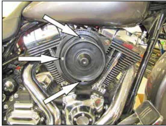
13. Install the K&N® air filter onto the back plate and secure with the provided hardware.
