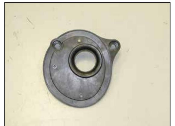
6. Install the provided venturi into the K&N<sup>®</sup> back plate as shown.
