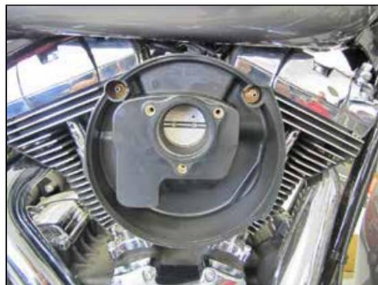
5. Remove the two breather bolts that secure the filter base to the engine and then remove the filter base from the engine.
