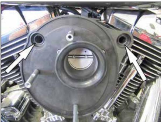
11. Install the two remaining O-rings into the back plate where shown.
