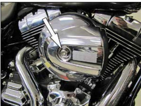
3. Remove the bolt that secures the bonnet to the air filter and then remove the bonnet.
