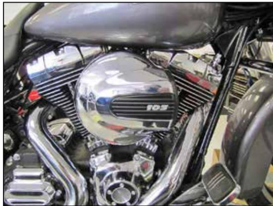
14. Install the factory bonnet onto the air filter and secure with the factory bolt. Install the decorative badge onto the bonnet.
