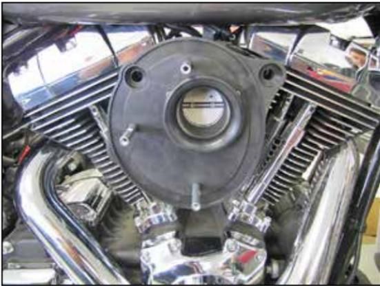
10. Place one drop of thread locker onto the three throttle body bolts and then install the back plate onto the throttle body and tighten the throttle body bolts.
