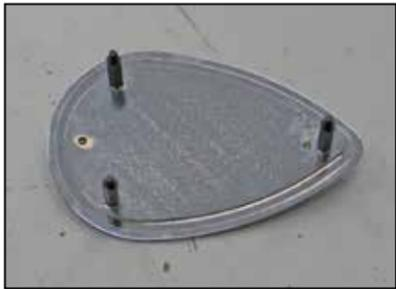
12. Apply thread locker to the three provided studs and then install the studs along with the lock washers onto the filter top plate as shown.
