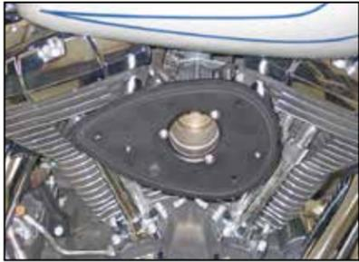
11. Install the three filter base plate mounting bolts into the base plate; install the remaining gasket and one drop of thread locker on each bolt. Secure the filter base plate to the Breather plate as shown.
