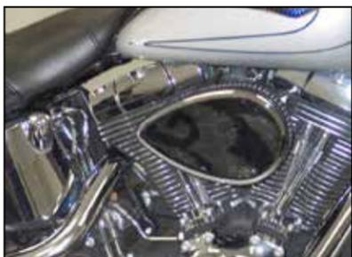
14. Install the filter/top plate assembly onto the base plate and secure with the provided hardware and thread locker.
