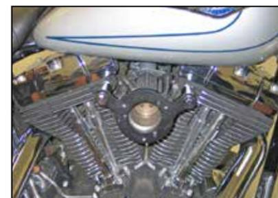
9. Install the crankcase breather plate along with the two remaining o-rings, mounting bolts (with one drop of thread locker) and throttle body gasket as shown.
