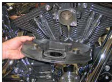
5. Remove the air filter base from the throttle body and unhook the wiring pig tail from the filter base.
