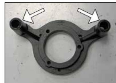
8. Install two of the provided o-rings into the crankcase breather plate as shown.
