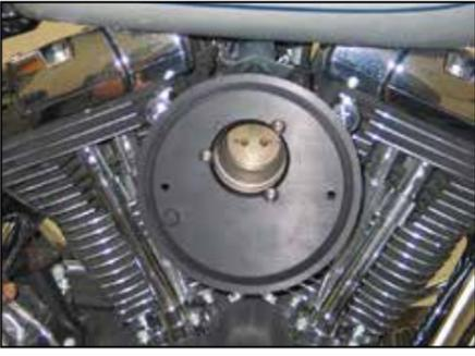
10. Install the three filter base plate mounting bolts into the base plate; install the remaining gasket and one drop of thread locker on each bolt. Secure the filter base plate to the breather plate as shown.
