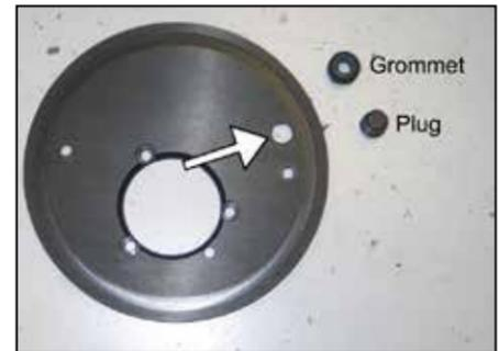
7. On vehicles equipped with a EVAP vent line, install the provided grommet into the hole shown. On vehicles not equipped with an EVAP vent line, install the provided plug into the hole shown from the back side of the base plate.
