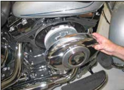
2. Remove the bolt which secures the bonnet to the filter assembly and then remove the bonnet from the vehicle.
