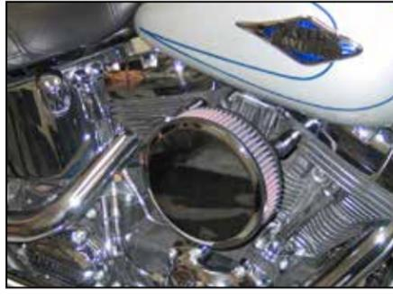
13. Install the filter/top plate assembly onto the base plate and secure with the provided hardware and thread locker.
