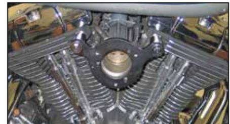
9. Install the crankcase breather plate along with the two remaining o-rings, mounting bolts (with one drop of thread locker) and throttle body gasket as shown.
