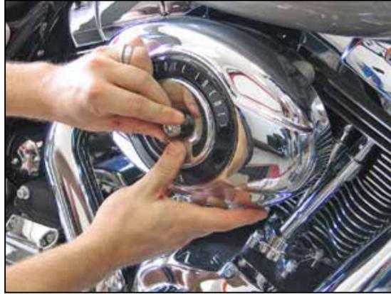
10. Install the bonnet onto the K&N® air filter and secure with the factory bolt.
