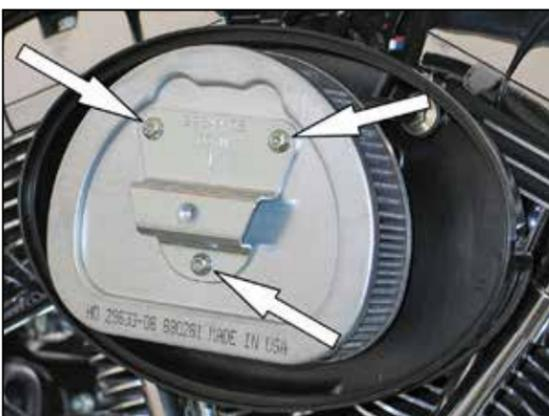
3. Remove the three bolts that secure the air filter and then remove the air filter and crank case breather tubes.
