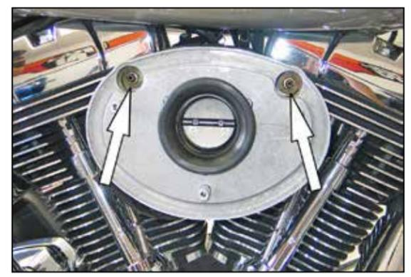
7. Install the filter back plate onto the throttle body and secure with the factory breather bolts and throttle body bolts provided. **NOTE: Be sure to install the two provided O-Rings into the receiver grooves on the back of the back plate.** **NOTE: On applications that have had the support bracket removed, install the two provided spacers between the back plate and cylinder head at the breather holes and then install the breather bolts as shown**
