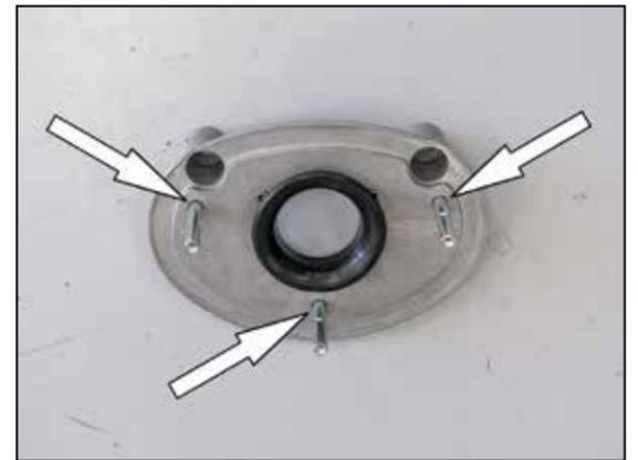
6. Install the three filter spacers onto the K&N back plate using the provided hardware. **NOTE: Be sure to place one drop of thread locker onto each bolt.**
