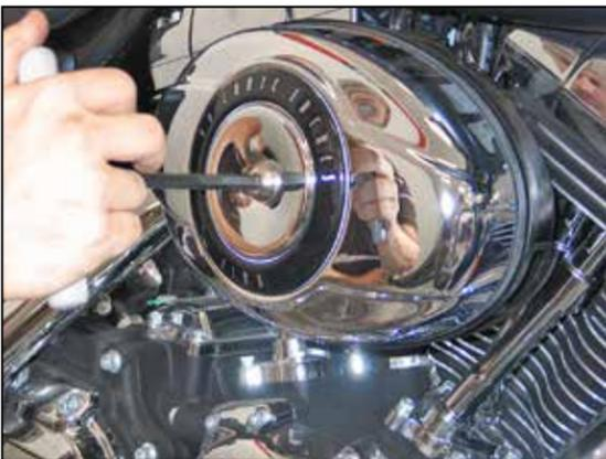
2. Remove the bolt securing the air filter bonnet and then remove the bonnet from the vehicle.
