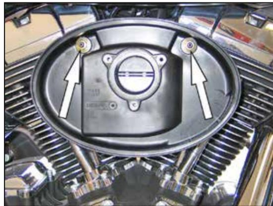
4. Remove the two crank case breather bolts securing the filter back plate and remove the back plate.
