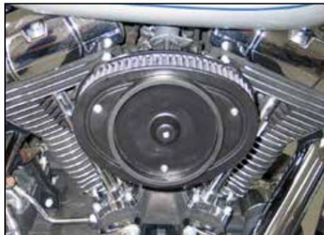
14. Install the air filter onto the base plate and secure with the three bolts provided.
