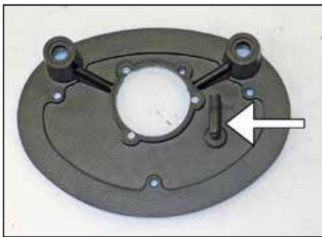
8. On models equipped with an EVAP vent line, drill a 1/2" id hole in the base plate at the location marked in step #7. Then install the provided grommet and 90° hose mender as shown.
