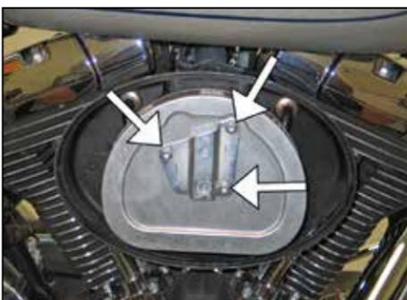
3. Remove the three bolts that secure the air filter to the filter base and remove the air filter along with the crank case breather tubes.
