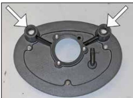
11. Install the two provided o-rings onto the base plate as shown.
