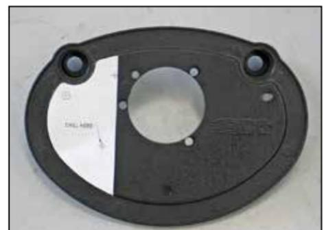
7. On models equipped with an EVAP vent line, cut out the provided template and place it on the filter base plate as shown. Mark the base plate for drilling a 1/2" ID hole.
