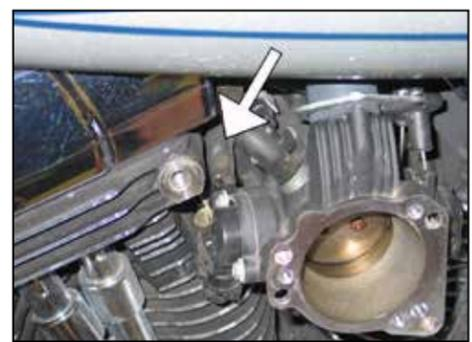
6. Using the provided tie wrap, secure the wiring pig tail to the throttle body wiring harness.
