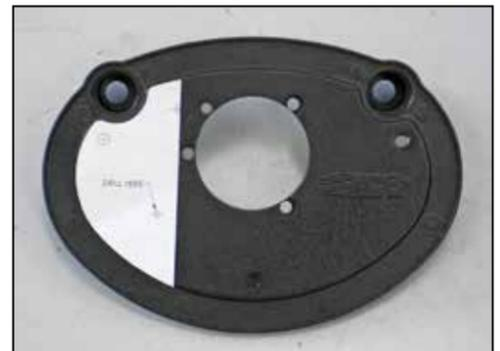
7. On models equipped with an EVAP vent line, cut out the provided template and place it on the filter base plate as shown. Mark the base plate for the 1/2"ID drill hole.
