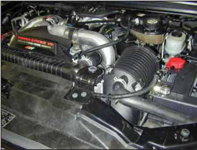
Factory air box system installed
