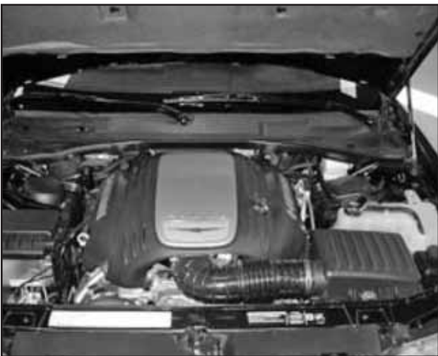
Factory air box system installed
