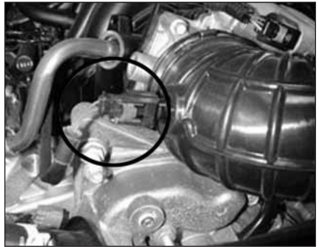
d. With the locking clip out, disconnect the IAT sensor wire harness from the sensor. Leave the IAT sensor in place.
