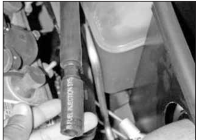
s. Insert the other end of the plastic connector into the factory crankcase breather hose.
