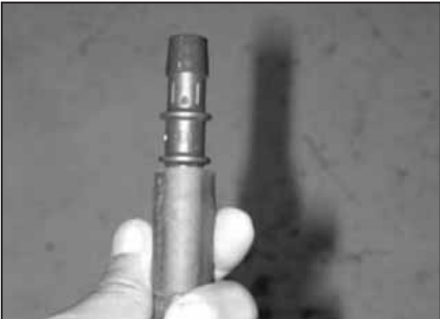
r. Insert the supplied plastic connector into the supplied breather hose.
