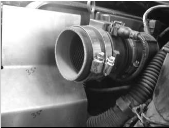
d. Attach coupler with supplied hose clamps.
