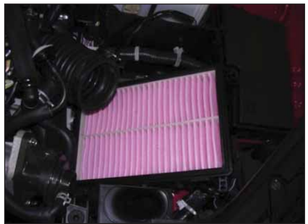
d. Unclip the two metal retaining straps securing the air filter housing lid to the lower airbox housing. Loosen the hose clamp securing the inlet tube to the turbo inlet pipe and remove the lid.
