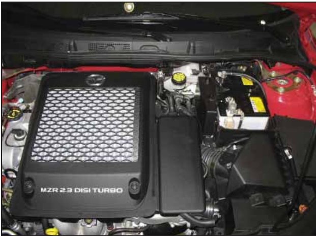
Factory airbox system installed
