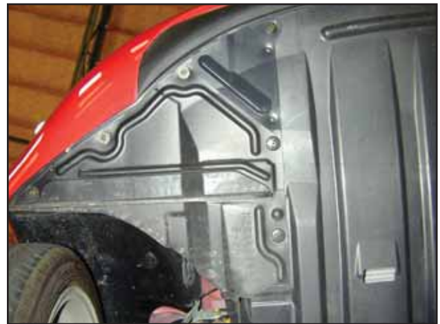
h. Remove the retaining clips and bolts securing the driver side splash shield to the bumper and chassis. Remove the splash shield.
