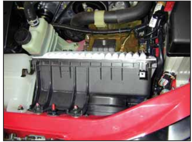
f. Remove the air filter housing lid by unhooking the metal retaining clips and sliding the lid out.
