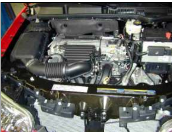
Factory air box system installed.
