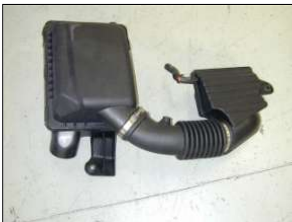
g. Remove the upper air box from vehicle.
