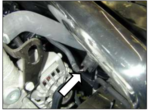
o. Insert IAT sensor through the grommet in the inlet pipe. Be careful not to push the grommet into the pipe.
