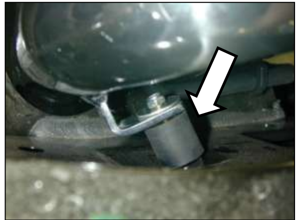
k. Place the inlet pipe support tab under washer as shown. Refer to step '3l' for proper installation.
