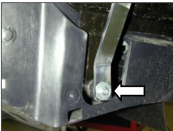
l. Place the lower support tab under the fender washer.
