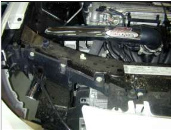
j. Install the intake pipe in engine bay as shown. Route the pipe up through the fender well into the engine bay.
