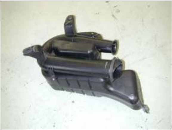
m. Remove the lower air box from the vehicle.
