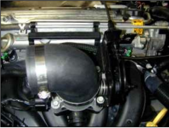
h. Install the rubber elbow onto the throttle body. Use the size 48 clamp at the throttle body. Do not tighten the clamp.
