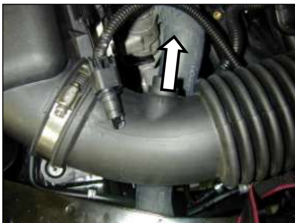
e. Gently pull out the inlet air temp (IAT) sensor from the rubber grommet.
