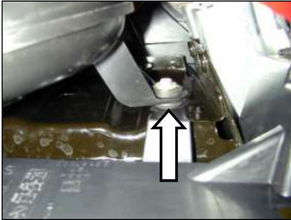
l. Loosen and remove the bolt securing the lower air box to the vehicle.
