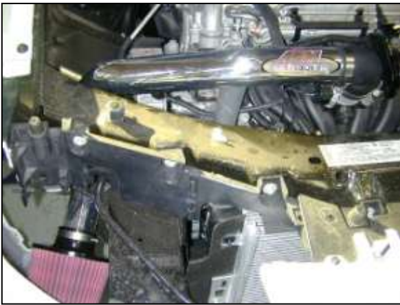
p. Install the air filter onto the end of the pipe.
