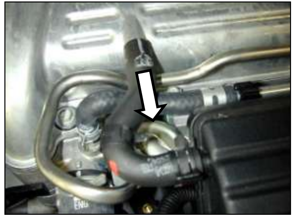
d. Release the spring clamp on the breather hose and pull hose off of the valve cover.
