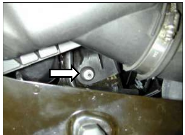
f. Remove the nut located behind headlight.
