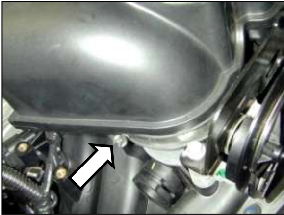
c. Loosen hose clamp at the throttle body.
