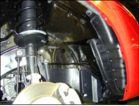
i. Release all the retainers and remove the fender liner from the fender well.
