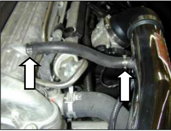
n. Install the supplied breather hose between the inlet pipe and valve cover. Secure it with the supplied 1" hose clamps.
