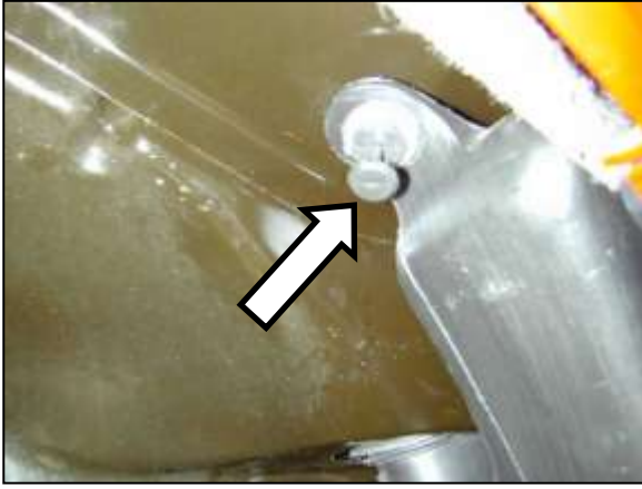
j. Release the upper retainer of the lower air box.
