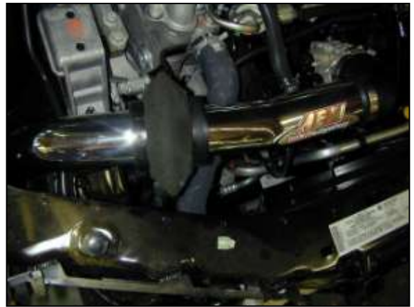
q. If an AEM ® bypass valve is installed, install the bypass valve as shown. The intake pipe will require some modification to accommodate the AEM bypass valve. Follow the instructions included with the bypass valve for proper installation.
