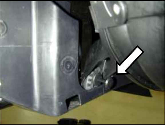
k. Remove the lower retainer of the lower air box.
