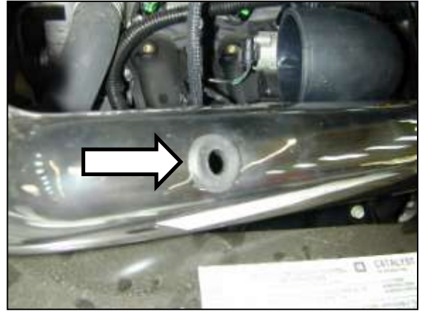
i. Insert supplied grommet into inlet pipe.
