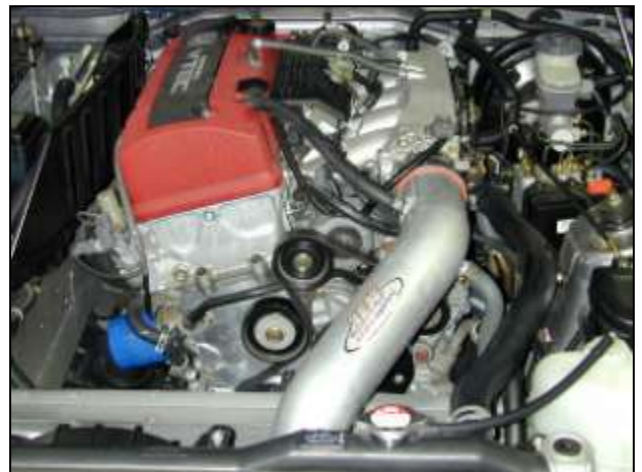
AEM® intake system installed
