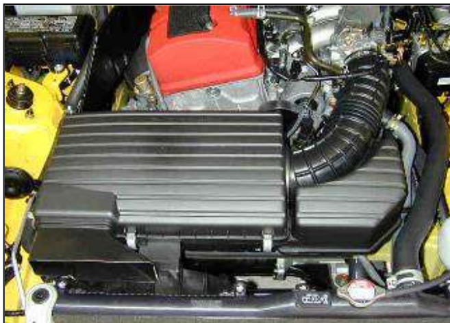
Factory air box system installed
