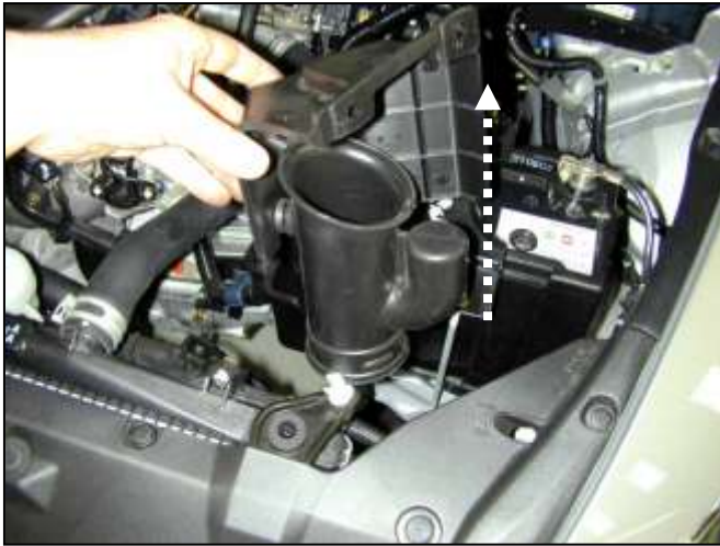
g. Pull upward on the plastic cover to remove the resonator box / intake tube.
