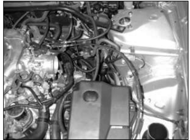
f. Remove air box assembly.
