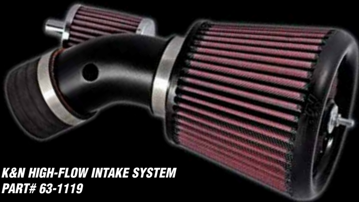
Powder-Coated Aluminum Intake Tube
