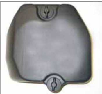
2. Loosen the air cleaner cover knobs and remove the cover.
