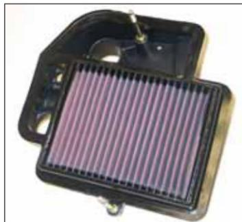
4. Install the K&N® air filter. Push down firmly so the rubber seal fits snugly along the grooves of the air box.
