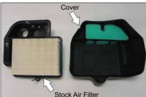
3. Remove the stock air filter with the integral rubber seal.
