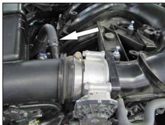
3. Release the spring clamp and disconnect the crank case vent hose from the factory intake tube.
