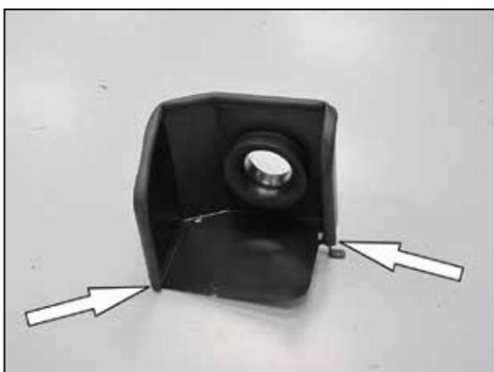
11. Install the provided edge trim onto the K&N® heat shield as shown.
