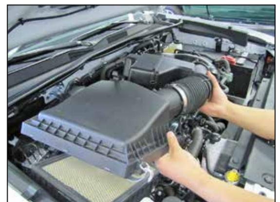
6. Release the two clips securing the air filter housing and then remove the intake tube and air filter hosing along with the factory air filter.
