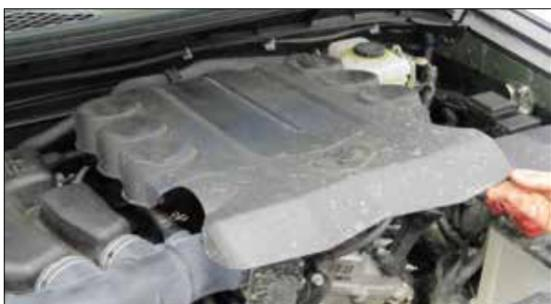
2. Lift up the engine cover to dislodge it from the mounting grommets and then remove the cover from the vehicle.
