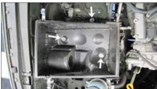
9. Loosen and remove the three bolts securing the lower air box and then remove the lower air box from the vehicle.
