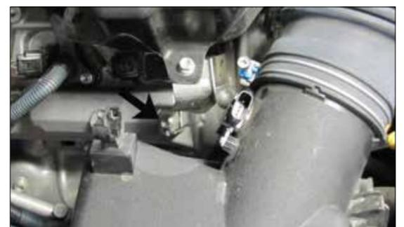
6. Remove the bolt which secures the tube mounting bracket to the engine valve cover.
