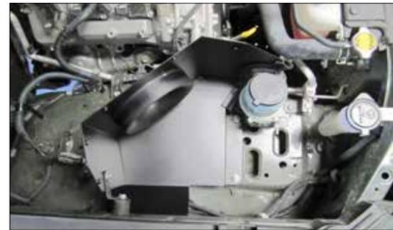
19. Set the heat shield onto the rubber mounted studs and secure with the provided hardware.
