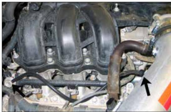
28. Connect the provided fuel pressure vent line to the fuel pressure regulator and then connect the open end to the 3/16 vent fitting in the K&N® intake tube.
