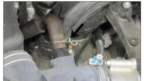
5. Disconnect the crank case vent hose from the stock intake tube.
