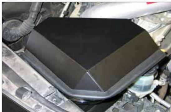
31. Install the heat shield cover onto the heat shield and secure with the provided hardware.
