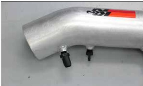
25. Install the 3/16 vent fitting into the K&N® intake tube as shown.
