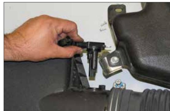
22. Remove the screws which secure the mass air sensor to the factory air box and then remove the mass air sensor from the air box.
