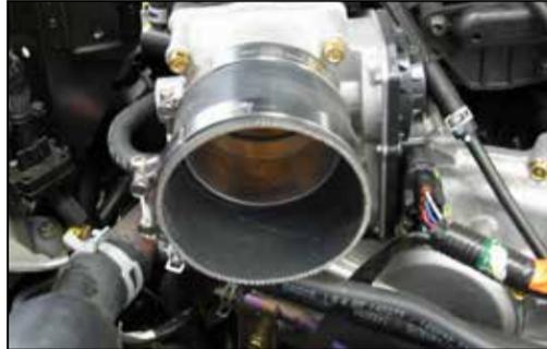
19. Install the silicone hose (084055) onto the throttle body and secure with the provided hose clamp.
