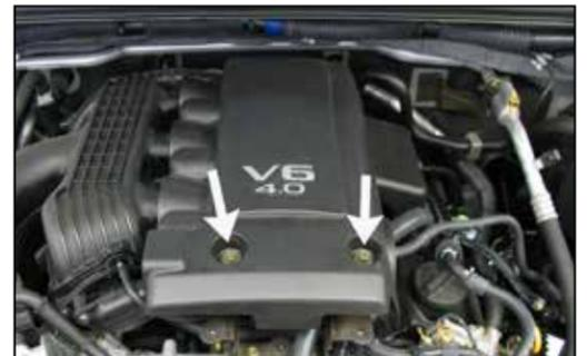
27. Reinstall the engine cover removed in step #4 and secure with the factory mounting bolts.
