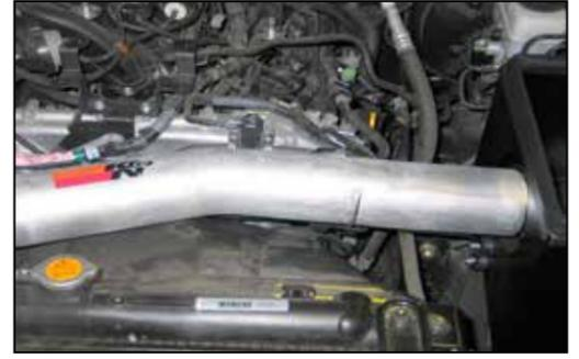
22. Install the K&N® intake tube into the silicone hose at the throttle body and align with the tube mounting bracket installed in step #16. Secure with the provided hardware and hose clamp.
