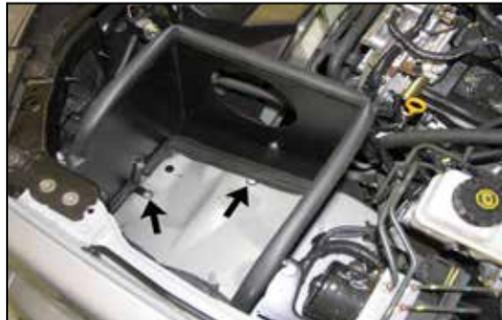
18. Install the heat shield assembly into the vehicle and secure with the provided hardware.
