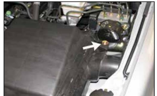
9. Remove the airbox retaining bolt shown.
