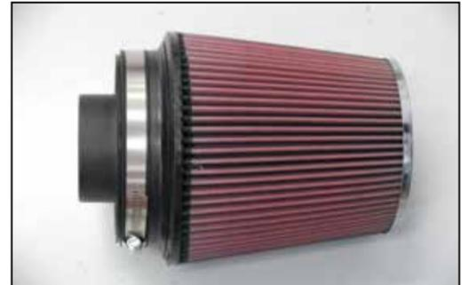
24. Install the filter adapter into the air filter as shown and secure with the provided hose clamp.
