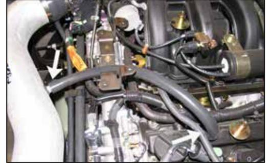
23. Attach the provided crank case vent hose to the valve cover and K&N® intake tube as shown and secure with the provided hose clamps.
