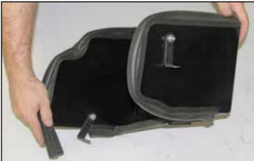
14. Install the edge trim onto the heat shield as shown.
