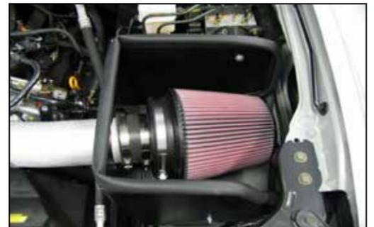
26. Install the air filter assembly onto the intake and secure with the provided hose clamp.
