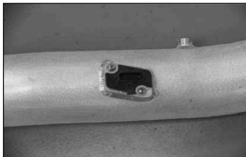
21. Install the mass air sensor into the K&N® intake tube and secure with the screws removed in step #20.
