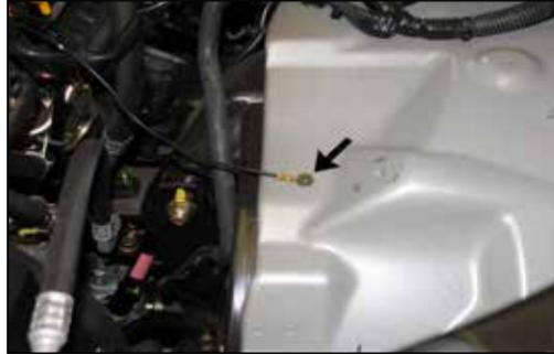
17. Remove the bolt, which secures the ground strap to the inner fender.
