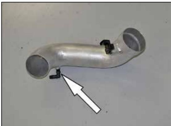
20. Install the provided 90° vent fitting into the K&N® intake tube as shown.
