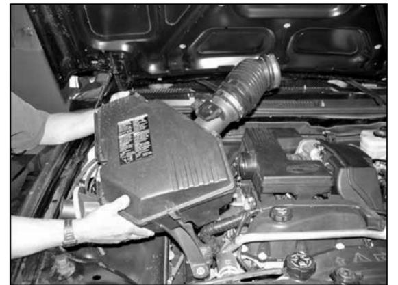
5. Lift up the air box and remove it from the vehicle. **NOTE: K&N recommends that customers do not discard factory air intake.**
