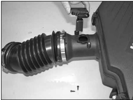
14. Remove the mass air sensor from the stock air box as shown.
