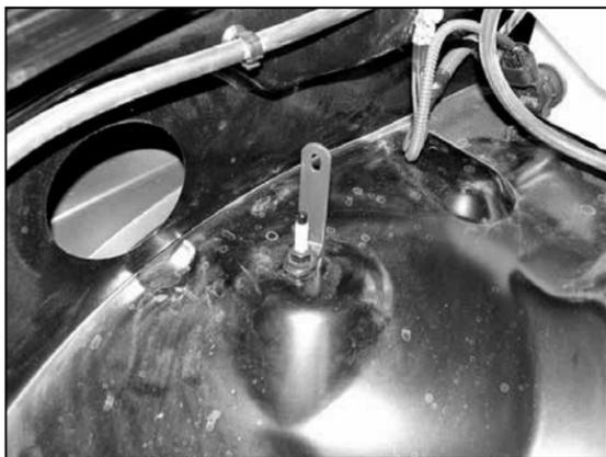
12. Install the "L" bracket (070602) onto the stock air box-mounting stud using the factory air box-retaining nut.
