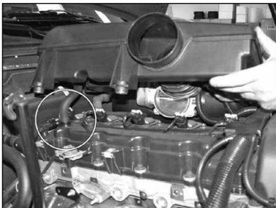
7. Remove the intake resonator from the engine as shown.
