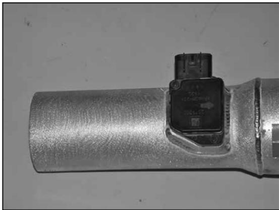
15. Install the mass air sensor into the K&N® intake tube using the factory bolts as shown.
