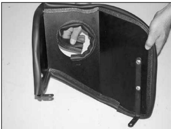
11. Install the edge trim onto the inner hole on the heat shield as shown. Trim if needed.
