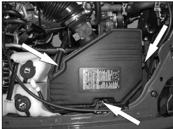
4. Loosen the two air box retaining bolts and one retaining nut.
