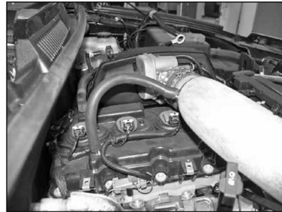
19. Install the provided crankcase vent hose onto the valve cover, then onto the K&N® intake tube as shown.
