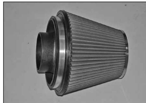
20. Install the filter adapter into the air filter and secure with the provided hose clamp.
