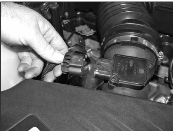
2. Depress the locking clip on the mass air sensor electrical connection, and then separate the mass air sensor electrical connection.
