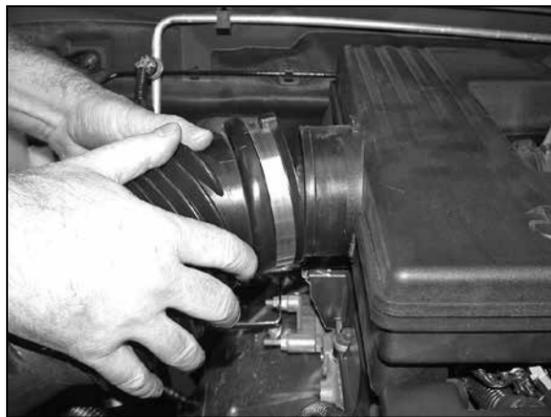
3. Loosen the hose clamp that retains the stock intake tube to the resonator, and then remove the tube from the resonator as shown.
