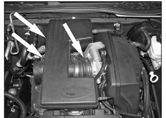
6. Loosen the two bolts that retain the intake resonator to the engine, and then loosen the hose clamp at the throttle body.
