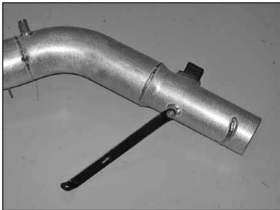
16. Install the small end of the tube-mounting bracket on the K&N® intake tube as shown.
