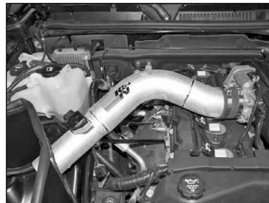
17. Install the K&N® intake tube into the silicone hose at the throttle body and through the heat shield, secure with the provided hose clamp.
