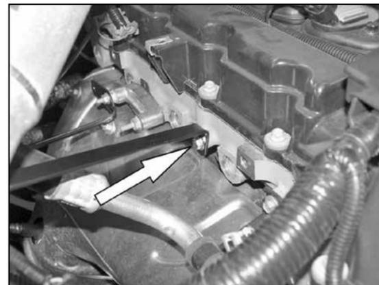
18. Attach the tube-mounting bracket to the engine using the provided hardware as shown.
