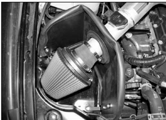
22. Install the air filter assembly onto the K&N® intake tube and secure with the provided hose clamp.
