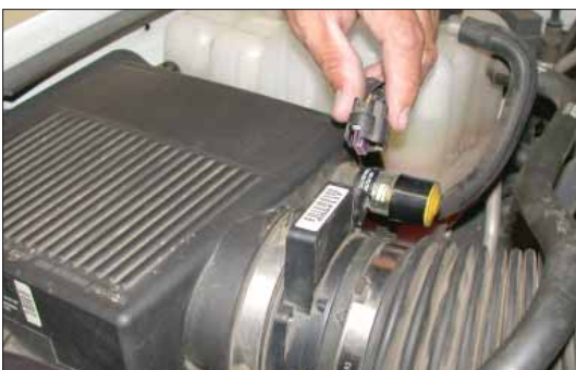
2. Disconnect the mass air sensor electrical connection as shown.
