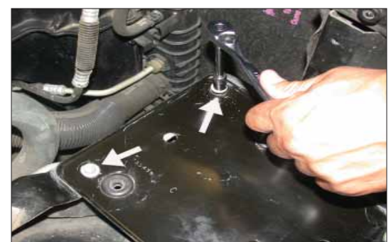
8. Remove the two stock air cleaner support tray bolts as shown.
