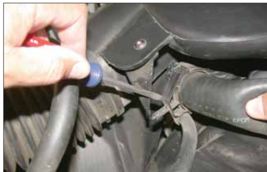
4. Unclip the radiator hose from the intake tube as shown.
