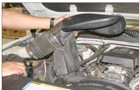
5. Disconnect the stock intake tube from the mass air sensor and from the throttle body, then, remove the intake tube as shown.
