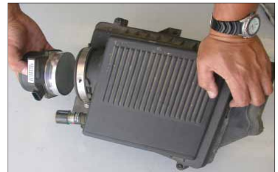
7. Loosen the hose clamp on the air cleaner then remove the mass air sensor as shown.
