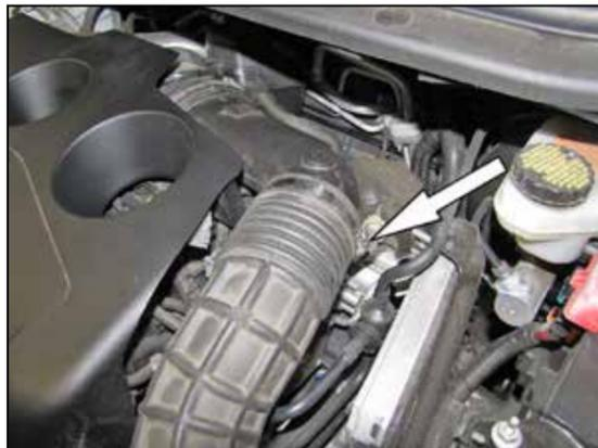
3. Loosen the hose clamp that secures the factory intake hose to the turbo inlet pipe.
