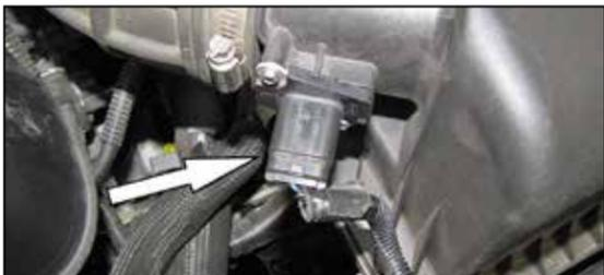
2. Release the locking tab and then disconnect the inlet air temperature sensor electrical connection and unhook the harness from the air filter housing.
