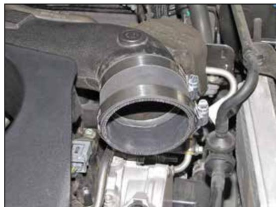
16. Install the appropriate coupling hose onto the turbo inlet pipe and secure with the provided hose clamp.
