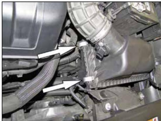
4. Release the two upper air filter housing retaining clips and then remove the upper air filter housing and intake hose assembly.
