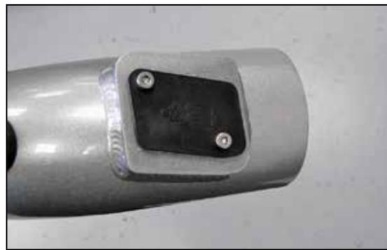
14c. Install the sensor block off plate with the provided gasket using the hardware provided.
