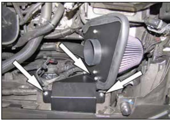
12. Secure the fresh air intake scoop to the core support and tighten the bolts which secure the scoop to the heat shield.
