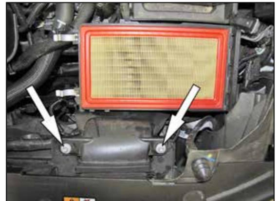
5. Remove the two bolts securing the fresh air intake scoop. Lift up the lower air filter housing to release it from the mounting grommets and then remove it from the vehicle.
