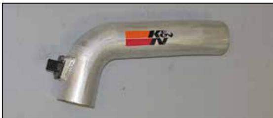
14. On vehicles equipped with the early style inlet temperature sensor, install the sensor into the K&N® intake tube and secure with the hardware provided.
