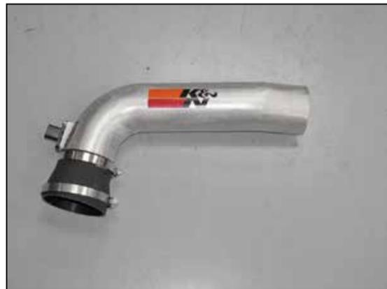
15. Install the step coupler hose (084055) onto the K&N® intake tube as shown. Do not tighten the hose clamp at this time.
