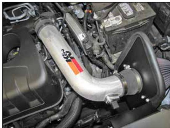
17. Install the K&N® intake tube assembly into the coupler at the turbo inlet tube, then slide the step coupler onto the filter adapter. Adjust the tube for best fit and secure the hose clamps.
