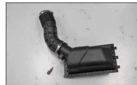
13. Remove the inlet temperature sensor from the factory air filter housing. The early style sensor requires removing the two screws that secure it. The later style requires lifting the locking tab and rotating the sensor counter clockwise while pulling out.
