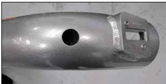
14a. On Vehicles equipped with the later style sensor, drill a 3/4" hole approximately 2" back from the sensor boss as shown. Be sure to remove any burrs caused during the drilling process. A Unibit will work well to drill the hole.
