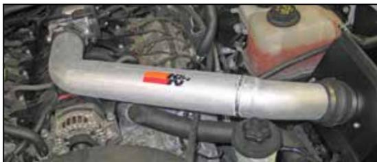
19. Install the K&N® intake tube into the silicone hose at the air filter and then into the silicone hose at the throttle body and secure with the provided hose clamps.
