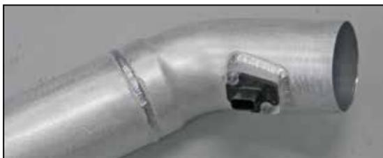
18. Install the mass air sensor into the K&N® intake tube and secure with the provided hardware.
