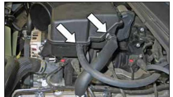
6. Disconnect the crank case vent line and EVAP vent line from the intake plenum.
