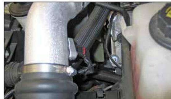
21. Reconnect the mass air sensor electrical connection.
