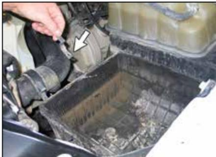
11. Remove the center air box lid mounting clip from the lower air box as shown.
