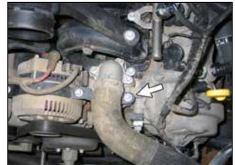
7. Remove the upper alternator mounting bolt shown. **NOTE: This bolt will be reused in the next step.**
