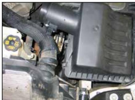
5. Release the three clips that secure the air box lid.
