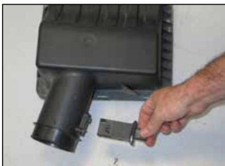
17. Remove the two screws securing the mass air sensor to the upper air box and then remove the mass air sensor from the upper air box.
