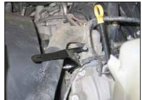
8. Install the tube mounting bracket (083111) and secure with the provided hardware and the bolt removed in the previous step.
