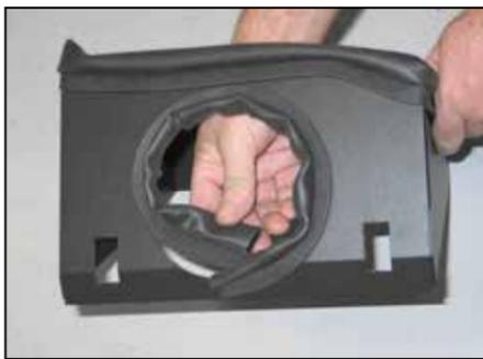
10. Install the provided edge trim into the hole in the heat shield as shown.
