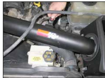
20. Connect the mass air sensor electrical connection.
