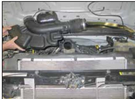
4. Remove the stock intake tube from the vehicle.
