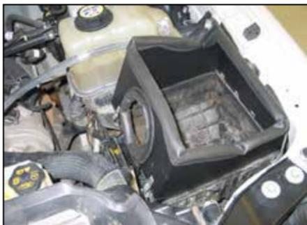
12. Install the heat shield assembly onto the lower air box and clip into place with the upper air box mounting clips.
