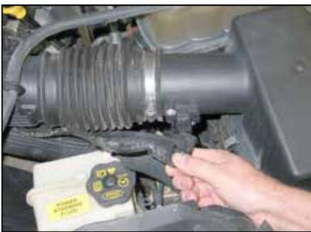
2. Release the red locking clip and then disconnect the mass air sensor electrical connection; unhook the wiring harness from the power steering reservoir.
