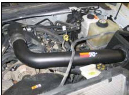
19. Place the K&N® intake tube through the heat shield, install the air filter assembly onto the end of the tube then install the intake tube into the silicone hose on the intake plenum. Secure the intake tube with the hardware and hose clamps provided.
