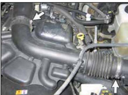
3. Loosen the hose clamps that secure the stock intake tube to the air filter housing and to the intake plenum.
