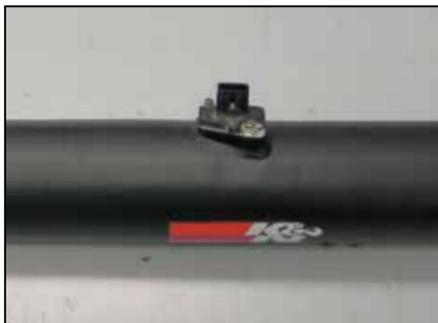
18. Install the mass air sensor into the K&N® intake tube and secure with the provided mounting screws.
