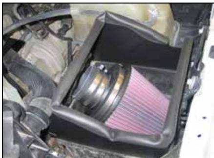
16. Place the filter assembly into the lower air box housing as shown.
