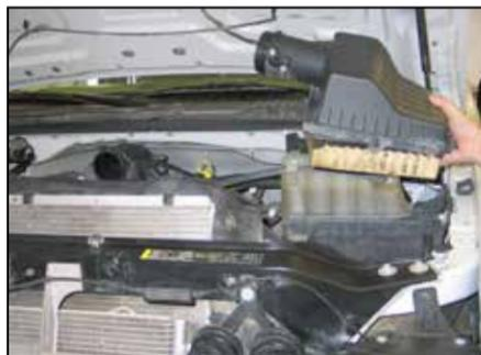
6. Remove the air box lid and stock air filter. **NOTE: K&N Engineering, Inc., recommends that customers do not discard factory air intake.**
