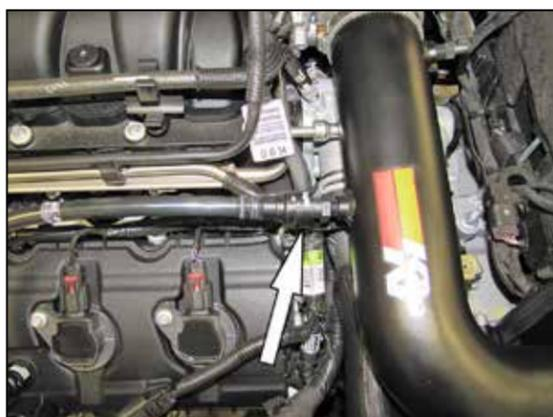
23. Connect the factory crank case vent to the quick connect fitting installed into the K&N® intake tube as shown.
