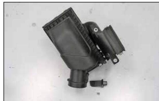
18. Remove the two screws that secure the mass air sensor into the factory air box and then remove the sensor from the air box.
