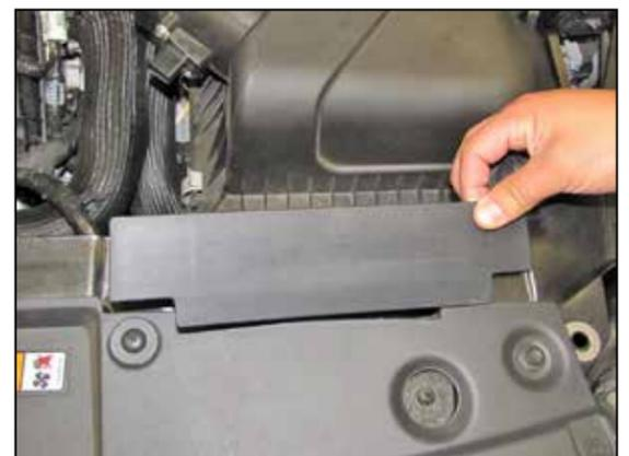
6. Remove the plastic cover over the fresh air intake scoop.
