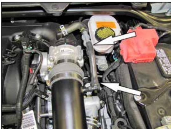
22. Using the provided hose, connect the EVAP vent line to the 90° vent fitting installed into the K&N® intake tube.
