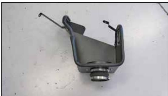
11. Install the provided hump coupler (08699) onto the filter adapter and secure with the provided hose clamp.
