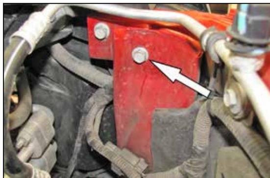
12. Remove the core support bolt shown.
