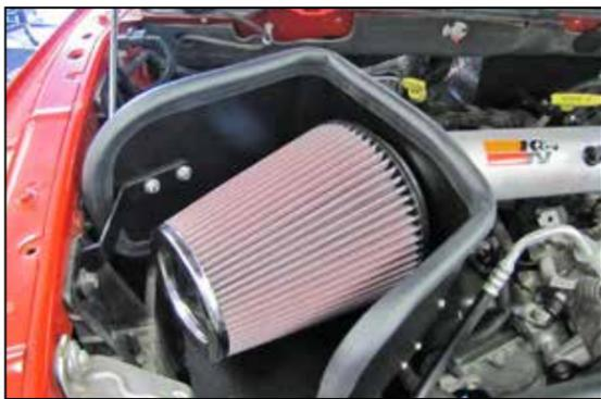
22. Install the K&N® air filter onto the adapter and secure with the provided hose clamp.
