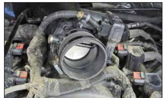
5. Install the provided coupling hose (08496) onto the throttle body and secure with the provided hose clamp.
