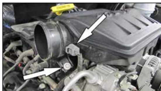
4. Disconnect the inlet air temperature sensor electrical connection and remove the bolt shown that secures the intake plenum. Lift up and remove the intake plenum from the vehicle.
