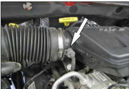
2. Loosen the hose securing the intake tube to the intake plenum.
