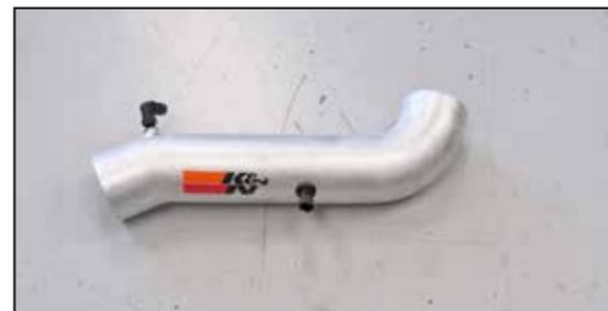
18. Remove the sealing O-ring from the sensor and then install the inlet air temperature sensor into the grommet installed into the intake tube.
