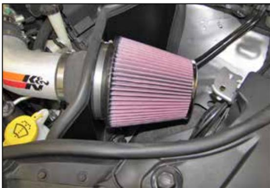
25. Install the K&N® air filter and secure with the provided hose clamp.
