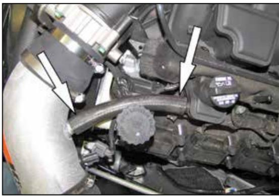
22. Install the provided crank case vent hose onto the valve cover port and then to the port on the K&N® intake tube.
