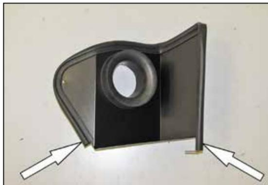
13. Install the edge trim onto the heat shield as shown.
