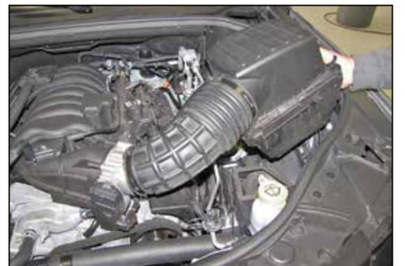
6. Lift up the air filter assembly to dislodge it from the mounting grommets and the remove the complete assembly from the vehicle.
