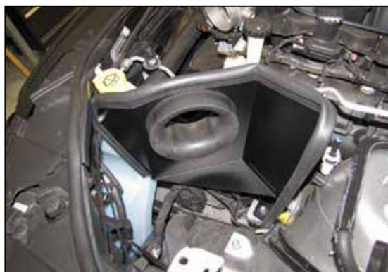
16. Install the heat shield assembly into the vehicle so the mounting grommet slides onto the inner most mounting stud. Align the heat shield with the mounting bracket and then secure with the spacer and hardware provided.
