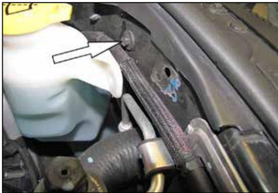
9. Remove the core support bolt shown.
