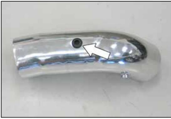
21. Install the provided grommet into the K&N® intake tube as shown.
