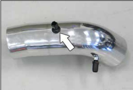
24. Install the inlet air temperature sensor into the grommet installed into the K&N® intake tube as shown.
