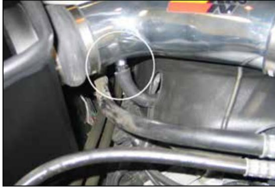
26. Connect the crank case vent hose to the fitting installed into the K&N® intake tube and secure with the provided hose clamp.
