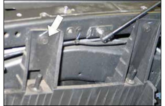
17. Remove the front air box mounting bracket bolt shown.
