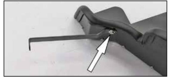
16. Install the heat shield mounting bracket (083103-1) onto the heat shield using the provided hardware.
