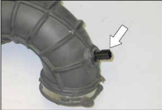
23. Remove the inlet air temperature sensor from the stock intake tube.
