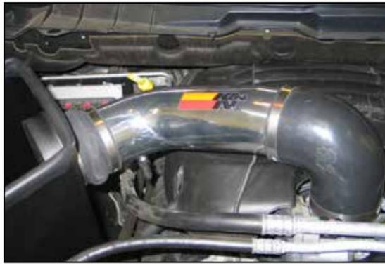
25. Install the K&N® intake tube into the silicone hump hose and then into the silicone hose attached to the throttle body. Align the heat shield assembly for proper fitment. Tighten the heat shield mounting bolts and hose clamps securing the intake tube.
