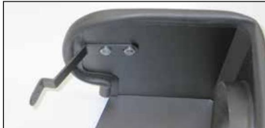
15. Install the heat shield mounting bracket (083127) onto the heat shield using the provided hardware.
