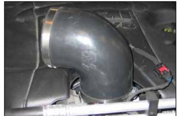
20. Install the provided silicone hose (084086) onto the throttle body and secure with the provided hose clamp.
