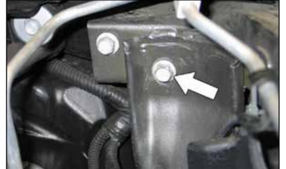
18. Remove the front fender mounting bolt shown.
