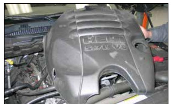
6. Lift up the engine cover to dislodge it from the mounting posts and then remove it from the vehicle.
