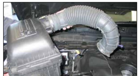
5. Disconnect the factory intake hose from the throttle body, then lift up the air box assembly and remove it from the vehicle.
