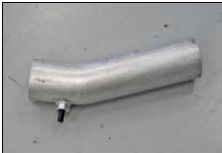
18. Install the inlet air temperature sensor into the K&N® intake tube as shown.
