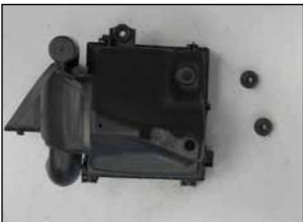
13. Remove two of the air box mounting grommets from the factory air box.
