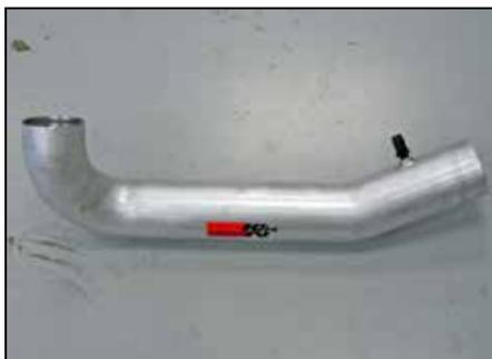
19. Install the provided ¼ npt vent fitting into the K&N® intake tube #27447 as shown.
