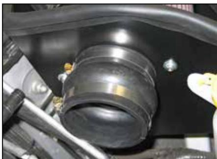
20. Install the provided hump hose (084057) onto to the filter adapter and secure with the provided hose clamp.
