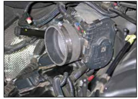
21. Install the provided silicone hose (08690) onto the throttle body and secure with the provided hose clamp.
