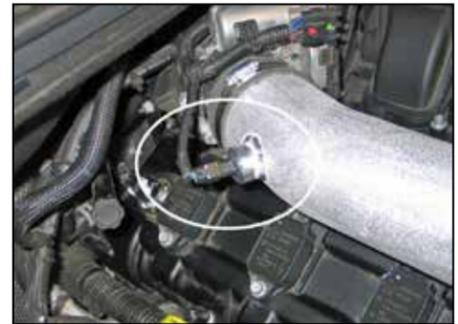
24. Reconnect the inlet air temperature sensor electrical connection.
