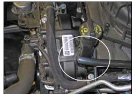
25. Measure the crank case vent tube 5" from the end and then cut off the end with a knife.
