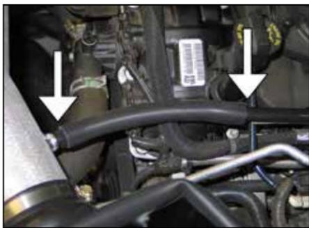
26. Install the provided crank case vent hose onto the vent fitting attached to the K&N® intake tube. Connect the open end of the crank case vent tube to the factory crank case vent tube that was cut in the previous step.
