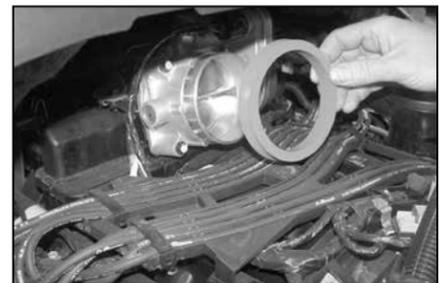
9. Remove the resonator silicone gasket from the throttle body.
