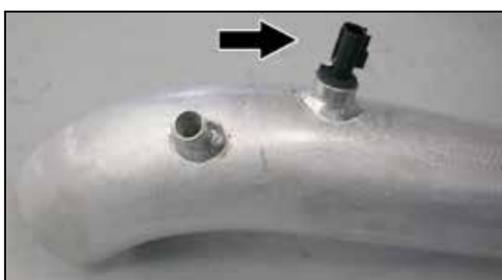
20. Install the air temperature sensor into the silicone hose on the intake tube as shown.
