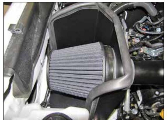
21. Install the K&N® air filter onto the filter adapter and secure with the provided hose clamp.
