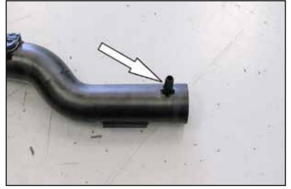
17. Install the provided NPT vent fitting into the K&N® intake tube as shown.
