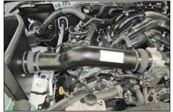
18. Install the intake tube into the coupling hose at the throttle body and then into the coupling at the filter adapter. Adjust the tube for best fit and then secure with the provided hose clamps.
