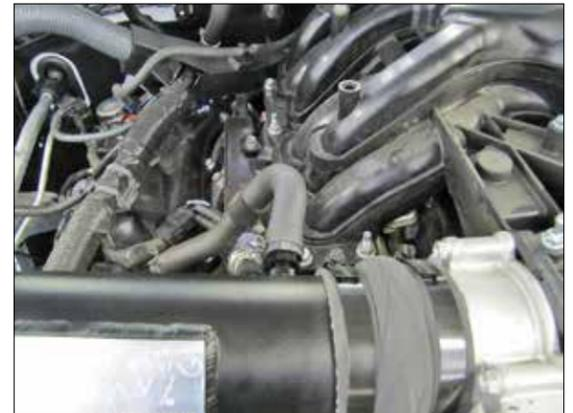
19. Connect the crank case vent fitting onto the vent fitting installed into the K&N® intake tube.
