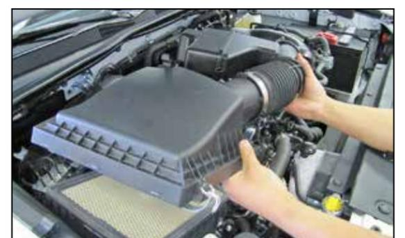
6. Release the two clips securing the air filter housing and then remove the intake tube and air filter hosing along with the factory air filter.
