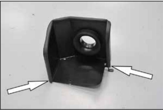
11. Install the provided edge trim onto the K&N® heat shield as shown.
