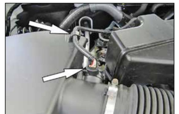
5. Disconnect the mass air sensor electrical connection and unhook the harness from the air filter housing.
