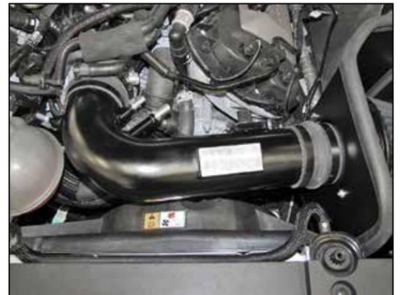
20. Install the K&N® intake tube into the hose at the filter adapter and then into the hose at the throttle body, adjust the tube and hoses for best fit and then secure with the provided hose clamps.
