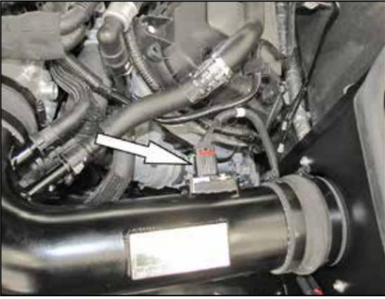
22. Connect the provided mass air sensor extension harness into the factory mass air sensor connection and then connect the other end to the mass air sensor.
