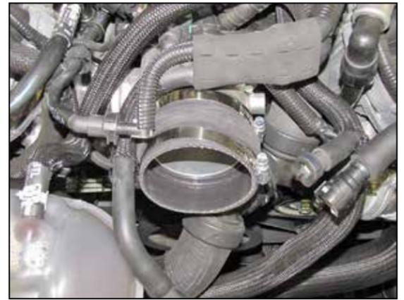
17. Install the provided hump coupler (08699) onto the throttle body and secure with the provided hose clamp.
