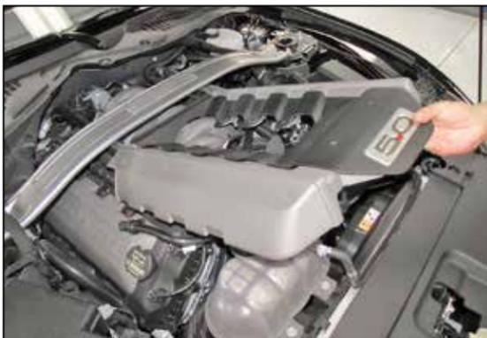
2. Lift up the decorative engine cover to dislodge it from the mounting studs and then remove the engine cover from the vehicle.
