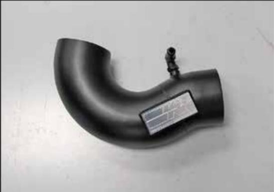
23. Install the provided 90° NPT fitting into the K&N® intake tube as shown.
