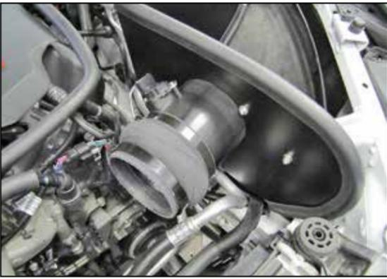
22. Install the provided step hump coupler (08633) onto the filter adapter and secure with the provided hose clamp.
