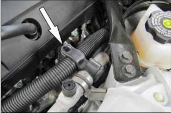
8. Disconnect the mount securing the sound tube to the A/C line.
