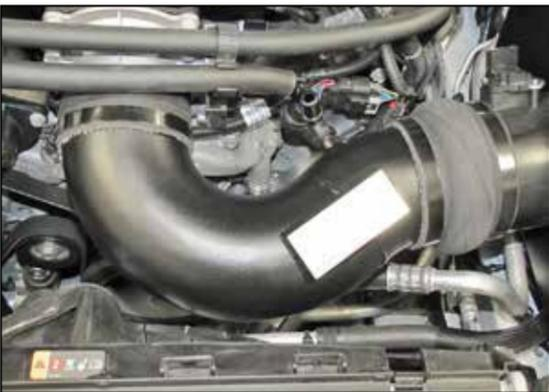
24. Install the K&N® intake tube into the hump coupler and then into the coupler at the throttle body, adjust the tube for best fit and then secure with the provided hose clamps.
