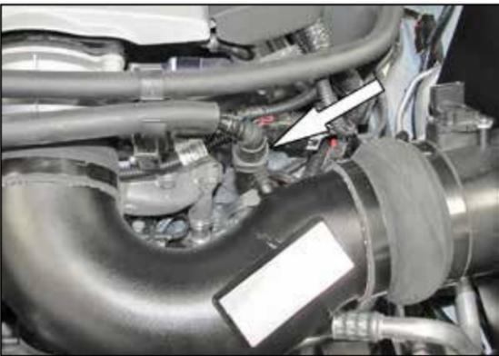
25. Connect the crank case vent hose to the quick disconnect fitting installed into the K&N® intake tube.
