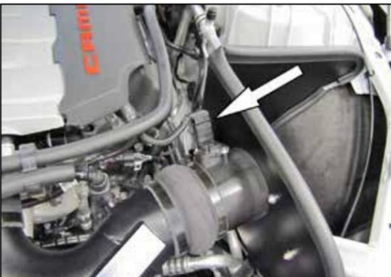
26. Connect the mass air sensor electrical connection.
