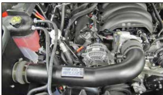
18. Install the K&N® intake tube into the hose at the filter adapter and then into the hose at the throttle body. Adjust the tube for proper fit and then secure with the provided hose clamps.
