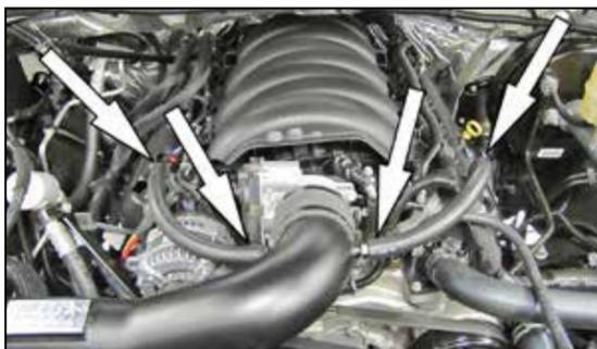
19. Install the provided crank case hoses onto the valve cover ports and then onto the fittings in the K&N® intake tube.
