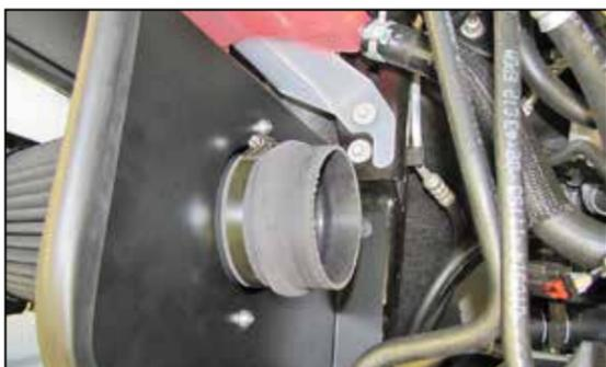
14. Install the provided coupling hose (08699) onto the filter adapter and secure with the provided hose clamp.
