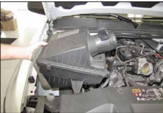
8. Pull firmly upward to release the air cleaner assembly from the mounting tray grommets. Then remove the assembly as shown.
