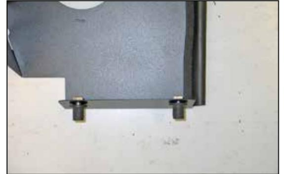
17. Install the remaining 5/16" inserted nut into the heat shield as shown.
