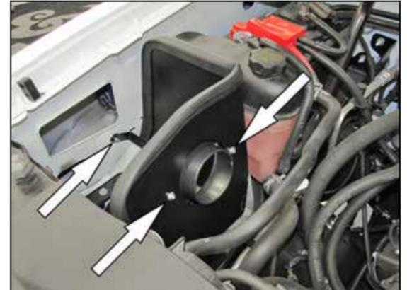
19. Secure the mounting bracket to the inner fender with the hardware provided. Then install the filter adapter onto the heat shield and secure with the provided hardware.
