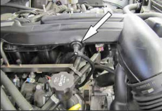
5. Unhook the crankcase vent line from the intake tube plenum as shown.
