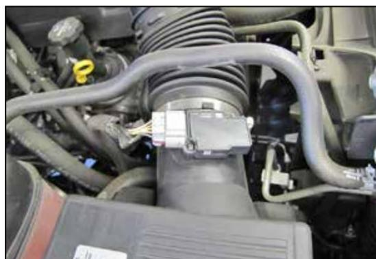
2. Disconnect the mass air electrical connection.
