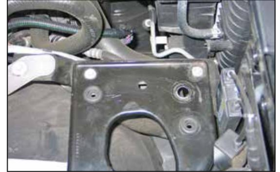
16. Remove the heat shield assembly and drill a 5/8" hole at the marked location.
