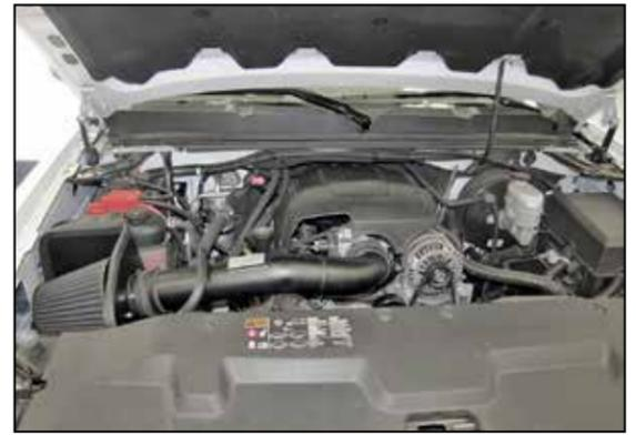
28. Reconnect the vehicle's negative battery cable. Double check to make sure everything is tight and properly positioned before starting the vehicle.
