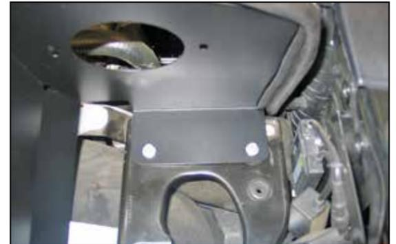
18. Reinstall the heat shield assembly onto the air box mounting plate and secure the two 5/16" bolts provided.
