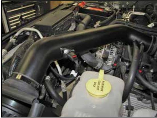
25. Connect the provided mass air sensor extension harness into the factory harness and then connect the open end to the mass air sensor.
