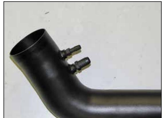
21. Install the two provided NPT vent fittings into the K&N® intake tube as shown.
