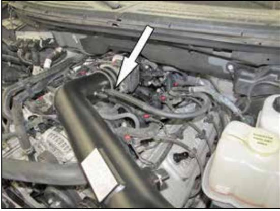
23. Install the provided hose mender into the provided EVAP hose and then install the hose mender into the factory EVAP hose. Connect the open end onto the fitting installed into the K&N® intake tube.
