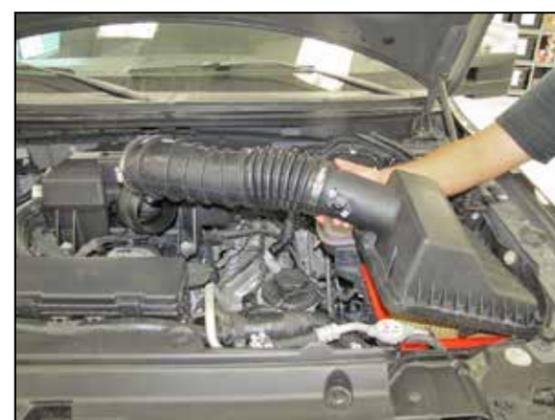
5. Remove the upper air box/intake hose assembly from the vehicle.
