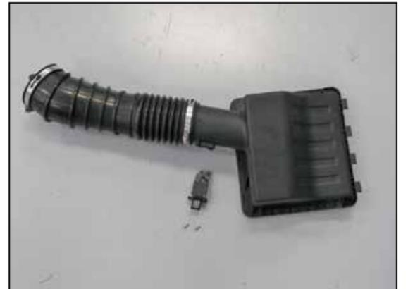
19. Remove the two screws securing the mass air sensor into the air box and then remove the sensor.
