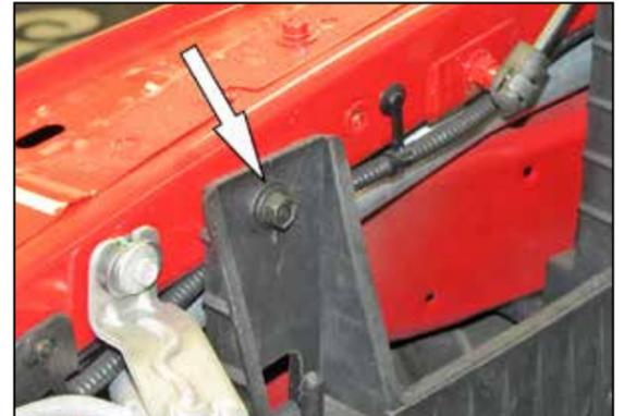
19. Remove the front air box mounting bracket bolt shown.
