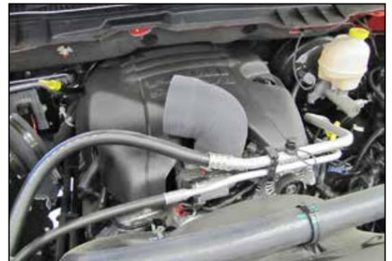
22. Install the provided silicone hose (08498) onto the throttle body and secure with the provided hose clamp.
