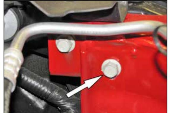
20. Remove the front fender mounting bolt shown.
