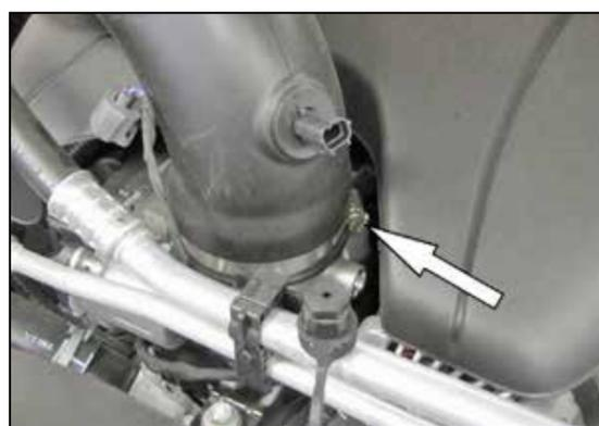
3. Loosen the hose clamp securing the factory intake tube to the throttle body.
