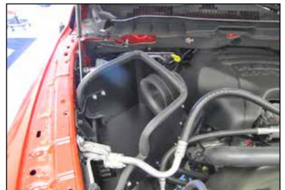
21. Install the heat shield into the vehicle and secure with the factory bolts from steps #19 and #20.
