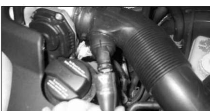
24. Remove the crank case vent hose from the intake hose as shown.
