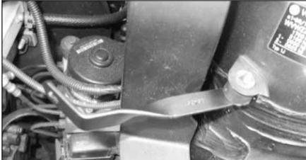
29. Screw the rubber vibration stud supplied into the original air box mounting point as shown, and mount the "L" bracket onto the stud using the M6 nut and waved washer supplied. Do not fully tighten yet!
