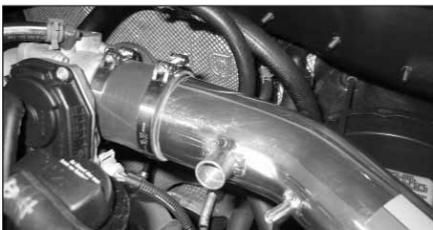
30. Slide the new intake tube into the silicone hose using the #300 barrel clamp supplied as shown. Don't fully tighten yet!
