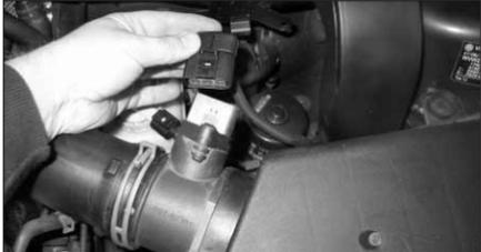
3. Disconnect the Mass Air Sensor (MAS) electrical connection as shown.
