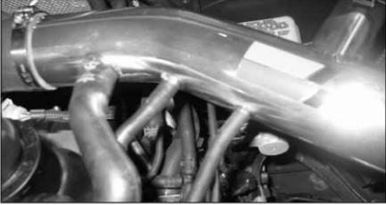
42. Refit the two vacuum hoses onto the intake tube as shown.
