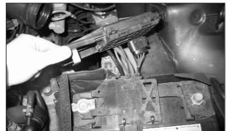
12. Disconnect the fuse/harness assembly from the positive battery terminal as shown.
