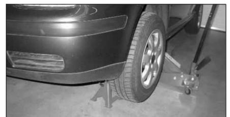
16. Taking all the necessary safety precautions lift the front of the vehicle upwards and support it with jack stands as shown.
