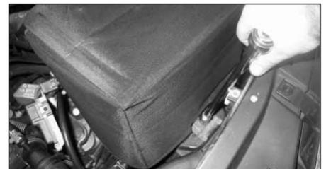
37. Reinstall the battery and the battery hold down block.
