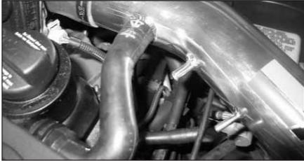
41. Fit the crank case vent hose onto the intake tube as shown.
