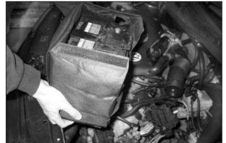
14. Remove the complete battery with the battery cover as shown.
