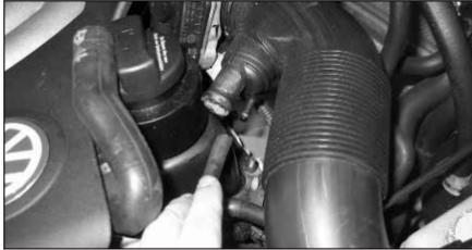
25. Remove the small vacuum hose underneath the crank case vent as shown.
