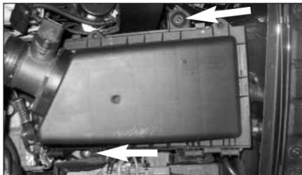
5. Remove the 2 airbox mounting bolts as shown.
