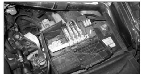
38. Reconnect the positive battery terminal and the fuse/harness assembly as shown.
