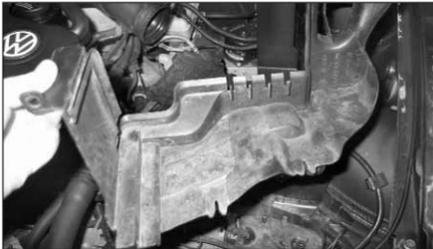
19. Remove the complete inner plastic headlight cover from the vehicle as shown.
