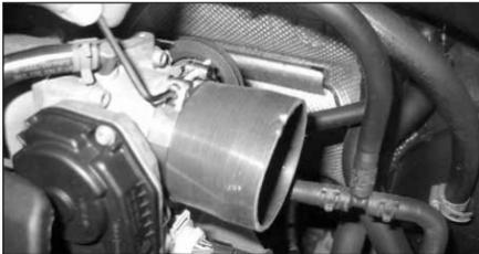
28. Fit a silicone stepped hose supplied onto the throttle body using the #275 barrel clamp supplied. To tighten, use the 9/64" Allen wrench supplied.
