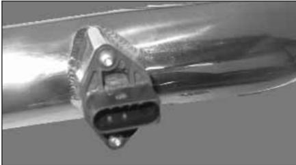
27. Mount the MAS onto the new intake tube using the two M5 bolts supplied.
