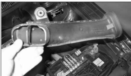
7. Remove the nut that secures the air inlet duct to the inner fender stud, then remove the inlet duct as shown. Attention: the nut will be re-used!
