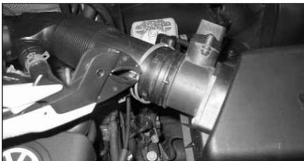
4. Carefully unclip the hose clamp from the MAS using a pair of pliers as shown.
