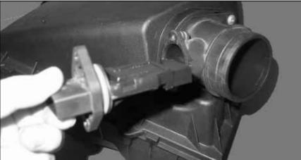
8. Unscrew and carefully remove the MAS from the airbox as shown.
