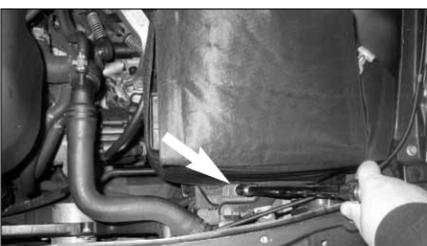
11. Remove the battery hold down block as shown.
