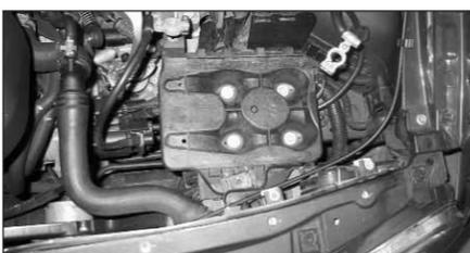
22. Reinstall the battery tray using the original four bolts.
