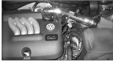
46. This K&N Typhoon intake kit has been designed to be used in two different configurations. In case of inclement weather, the cold air tube can be removed and the filter can be clamped onto the first intake tube located in the engine compartment as shown to avoid the possibility of ingesting water into the engine.
