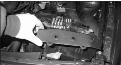
9. Remove the outer core support cover, which is secured by two screws.
