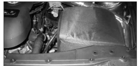
39. Reconnect the negative battery terminal, the battery cover and the two core support covers as shown.
