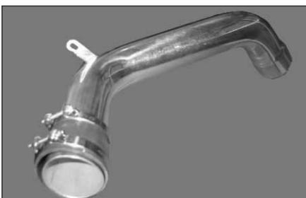
32. Install a silicone hose and the two barrel clamps onto the cold air extension tube as shown. Make sure to fit the hose over the non-swaged end of the tube & don't fully tighten yet!
