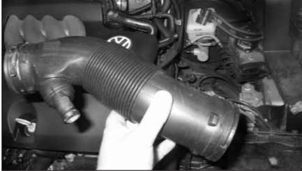
26. Undo the clamp and remove the complete intake hose from the vehicle as shown.
