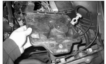
15. Remove the battery tray which is secured by four bolts.
