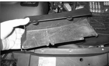
10. Remove the inner core support cover, which is secured by two screws.
