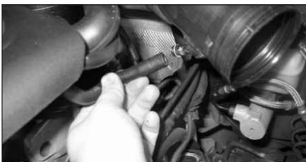
23. Remove the small vacuum hose from the intake hose as shown.
