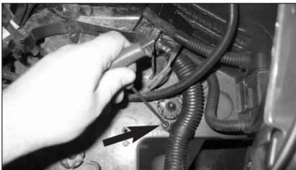
21. Using the provided plastic clamp secure the harness to the inner fender using the M5 hardware supplied.
