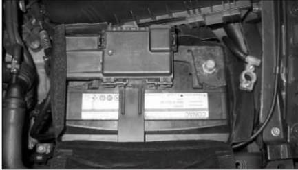
2. Remove the battery cover and disconnect the negative battery terminal.
