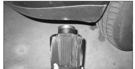
36. From underneath the vehicle install the filter onto the cold air tube using the hose clamp supplied.
