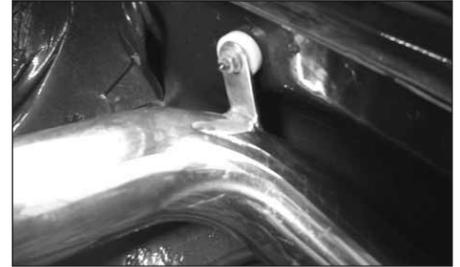
33. Fit the nylon spacer supplied over the stud on the inner fender. Now feed the swaged end of the cold air extension tube into the hole in the inner fender, then line up the bracket with the stud as shown and secure with the nut removed in step 7. Don't fully tighten yet!
