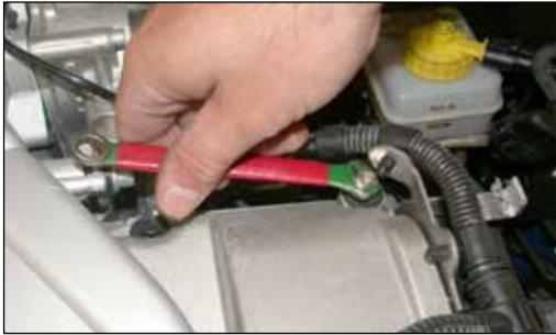
11. Loosen the nut on the cam cover but do not remove as shown.
