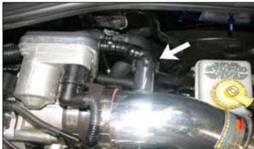
21. Reconnect the crank case vent hose to the vent on the K&N® intake tube.
