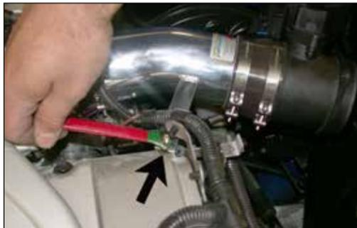
19. Adjust the tube for best fit and clearance and tighten the nut on the cam cover as well as the hose clamps on the intake tube as shown.
