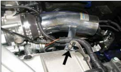
13. Slide the intake tube into the silicone hose on the throttle body, then, line up the bracket with the stud from step 11 as shown.
