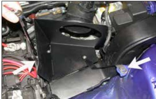
18. Install the heat shield into the vehicle and secure it using the stock air cleaner bolts, adjust for best fit and clearance and tighten all hardware.
