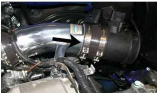
15. Slide the mass air assembly onto the K&N intake tube, but do not tighten at this time.
