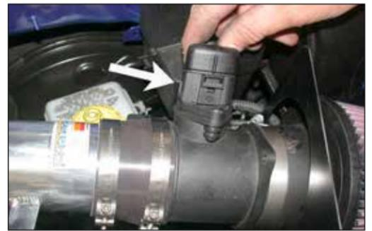
22. Reconnect the mass air sensor electrical connection as shown.
