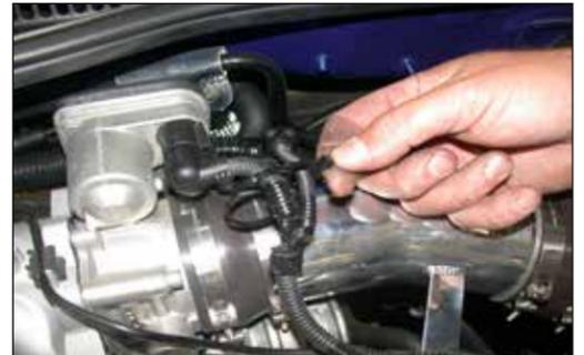
23. Zip-tie the crank case vent switch to the throttle control connection as shown.
