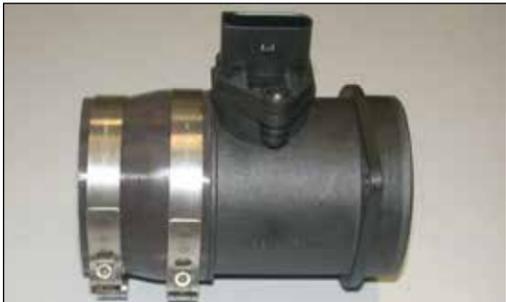
14. Install the silicone hose and hose clamps onto the mass air sensor as shown.
