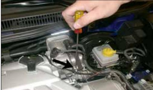
12. Install the silicone hose and hose clamps onto the throttle body as shown.
