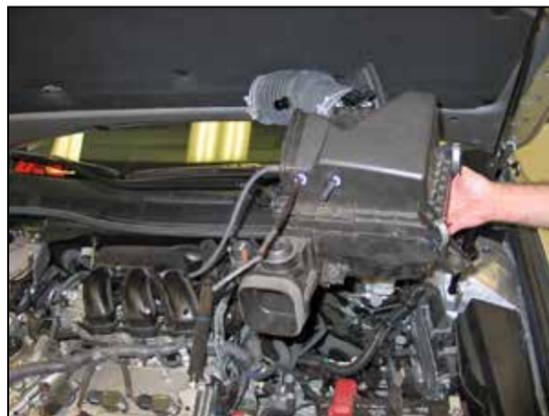
15. Remove the air box from the vehicle.
