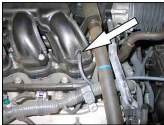
3. Disconnect the vacuum line shown from the intake plenum.
