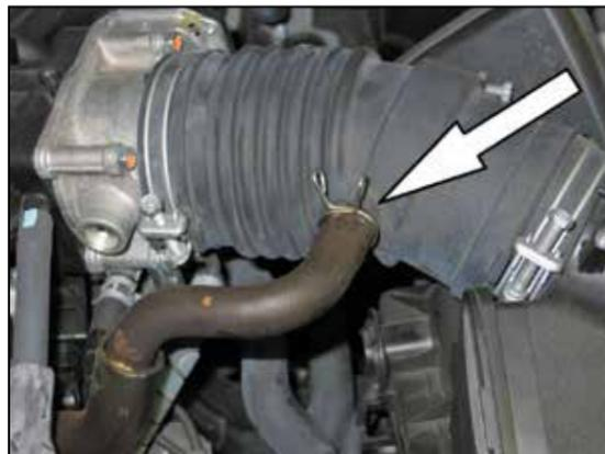
4. Disconnect the crank case vent hose from the intake tube.
