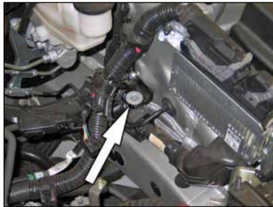
16. Remove the air box mounting grommet shown.
