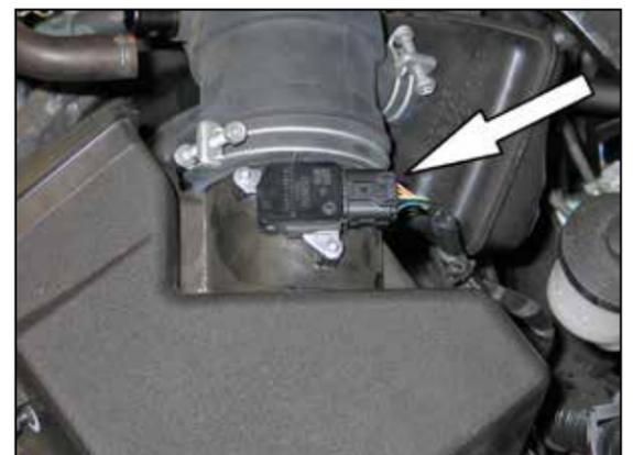
6. Disconnect the mass air sensor electrical connection and then unhook the wiring harness from the air box.
