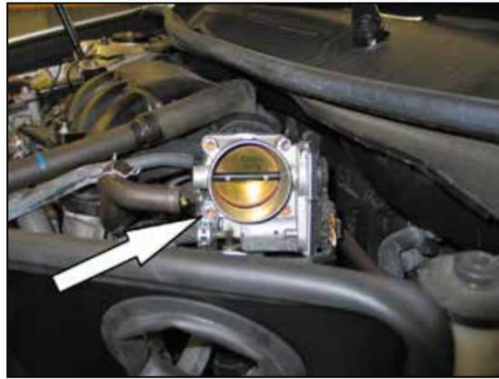
27. Remove the front lower throttle body mounting bolt shown.
