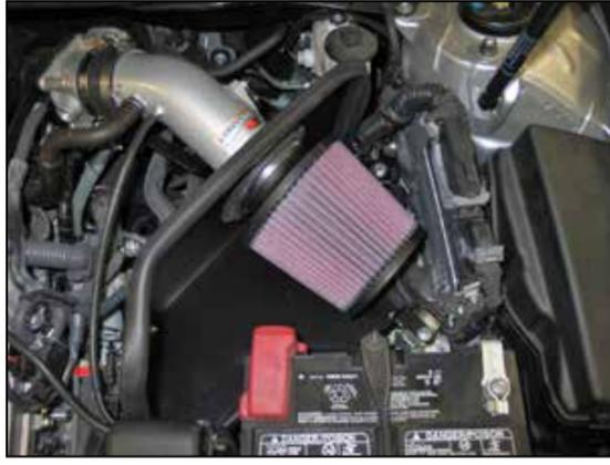
41. Install the K&N® air filter and secure with the provided hose clamp.
