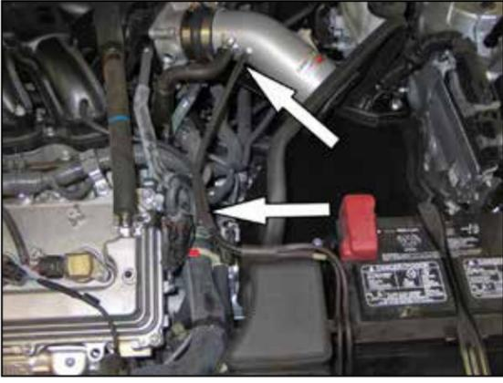
37. Connect the shorter provided vacuum line to the open factory union fitting and then connect the open end to the K&N® intake tube.
